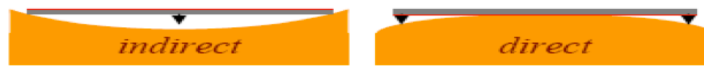
Figure 54: Two possible setups for the hot slumping of a glass, with the direct and indirect method where the optical surface in contact (or not) with the mould [Illustration by Ghigo et al., 2009].
