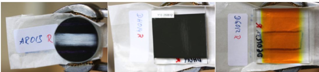
Figure 71: Coating samples after a severe abrasion test. Upper: Al + SiO 2 . Middle: Al + SiO 2 + HfO 2 + SiO 2 . Lower: dielectric coating [Förster, 2013].
