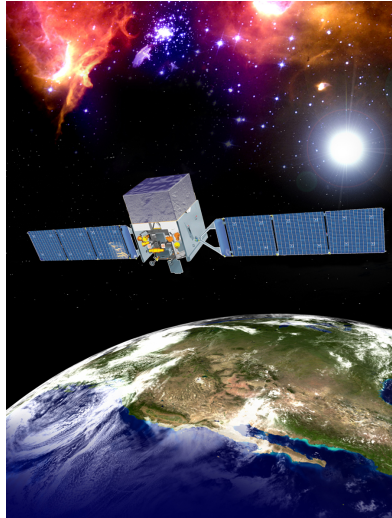
Figure 16: Artistic image of the FERMI spacecraft. The LAT detector is visible on top. Its effective area is \sim 1 \text{ m}^2 .
