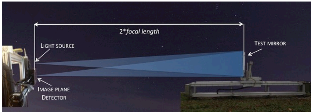
Figure 80: Optical set-up for the 2f configuration.
