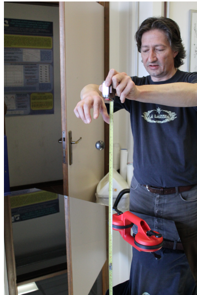
Figure 74: Impact test on a MAGIC mirror. Courtesy of M. Mariotti.
