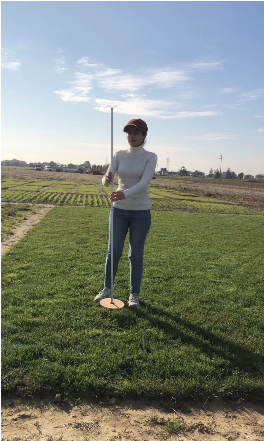
Figure 1. Measurement of turfgrass height prior to mowing using a grass plate meter
