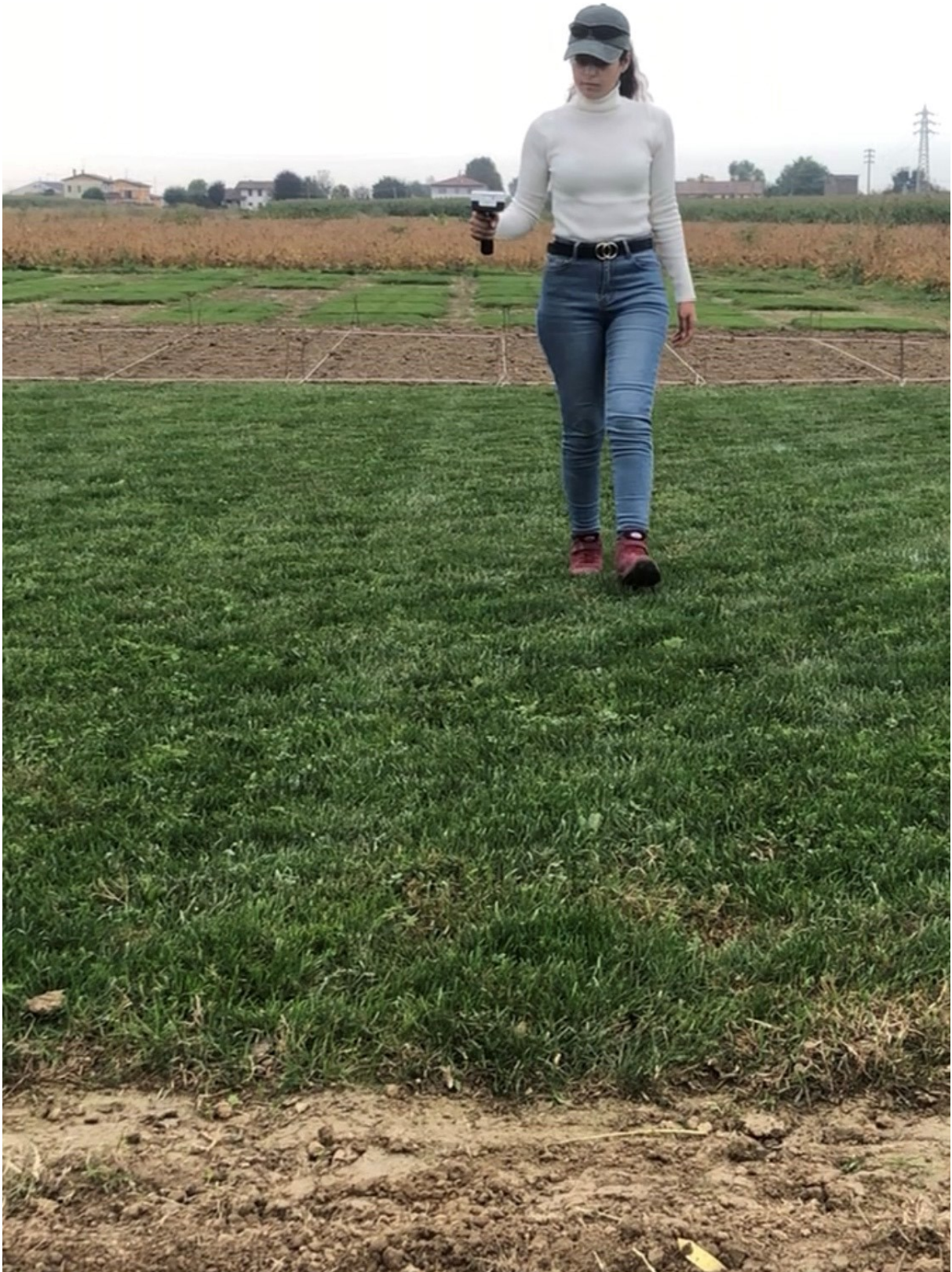
Figure 4. Using the NDVI with the RapidSCAN CS-45 to assess the physiological condition of the turfgrass and monitor its overall health
