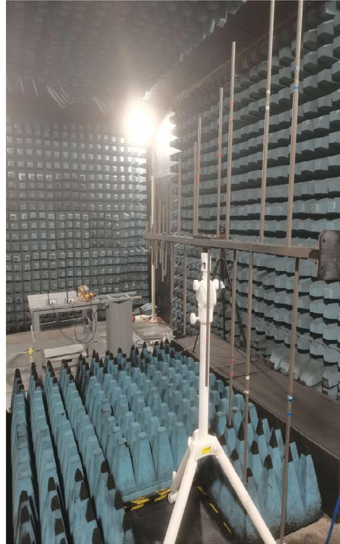
Figura 14: setup camera anecoica.
