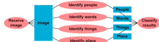
(b) Example of task parallelism applied to an image: multiple war tasks are executed in parallel and each task is executed in parallel does something different.
