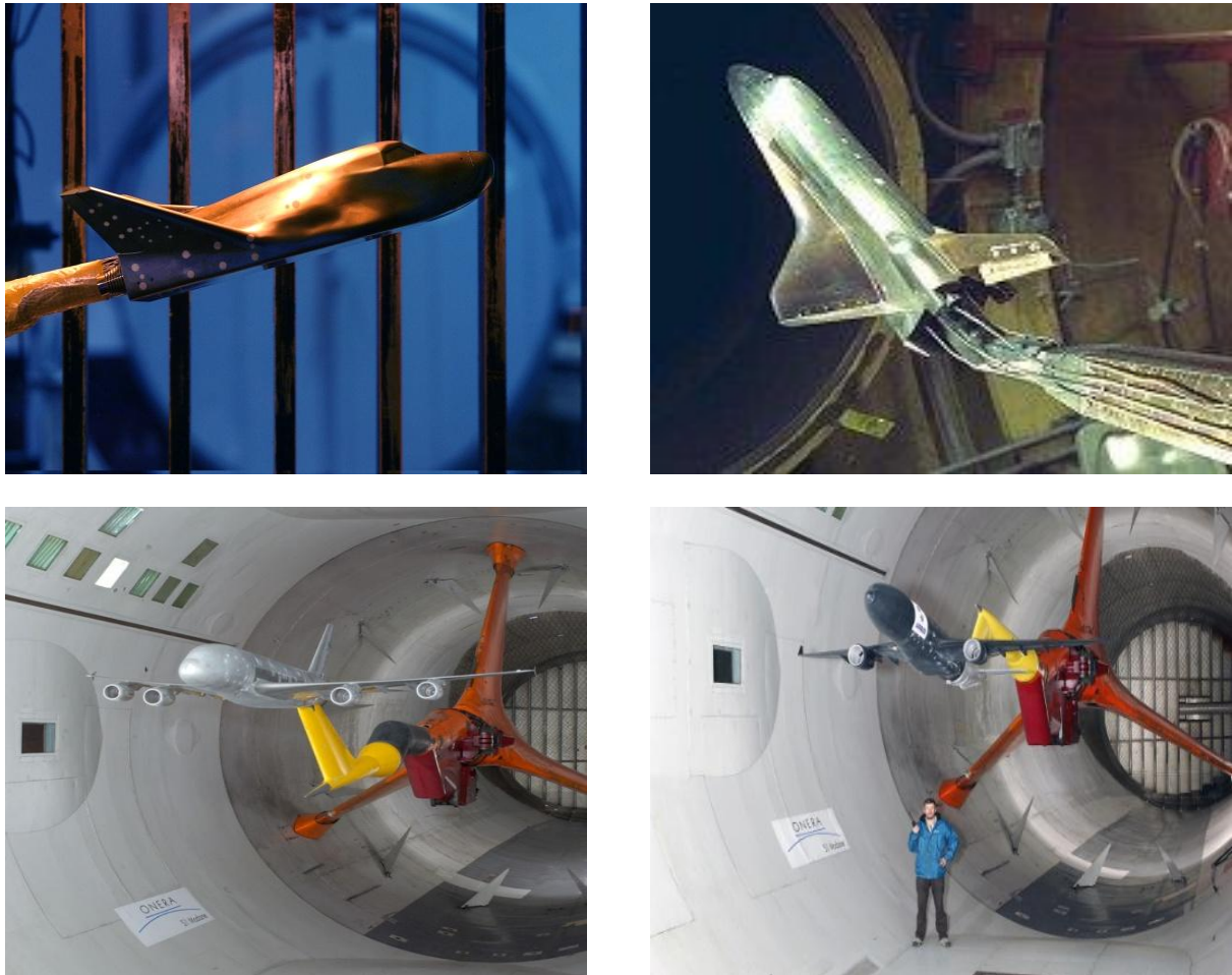
Figure 12. On the top left the Dream chaser with a rectilinear sting, on the right the Shuttle with a bent sting. On the bottom left a "Z sting", while on the right a "fin sting" both applied at commercial planes (ONERA S1MA wind tunnel).
