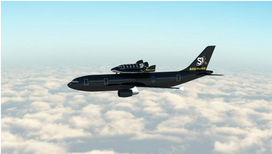
Figure 2. SOAR and Airbus carrier in the composite configuration before the separation.
