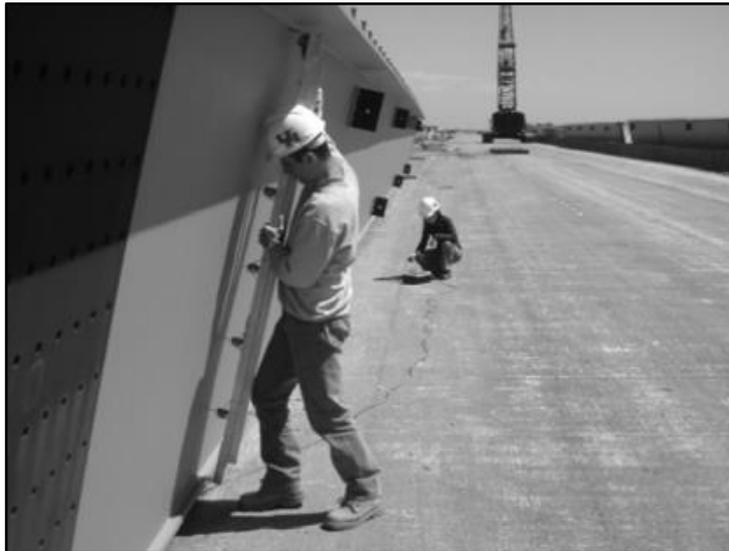
**Figure 1.14.** Measurements of web imperfections with dial gauges
