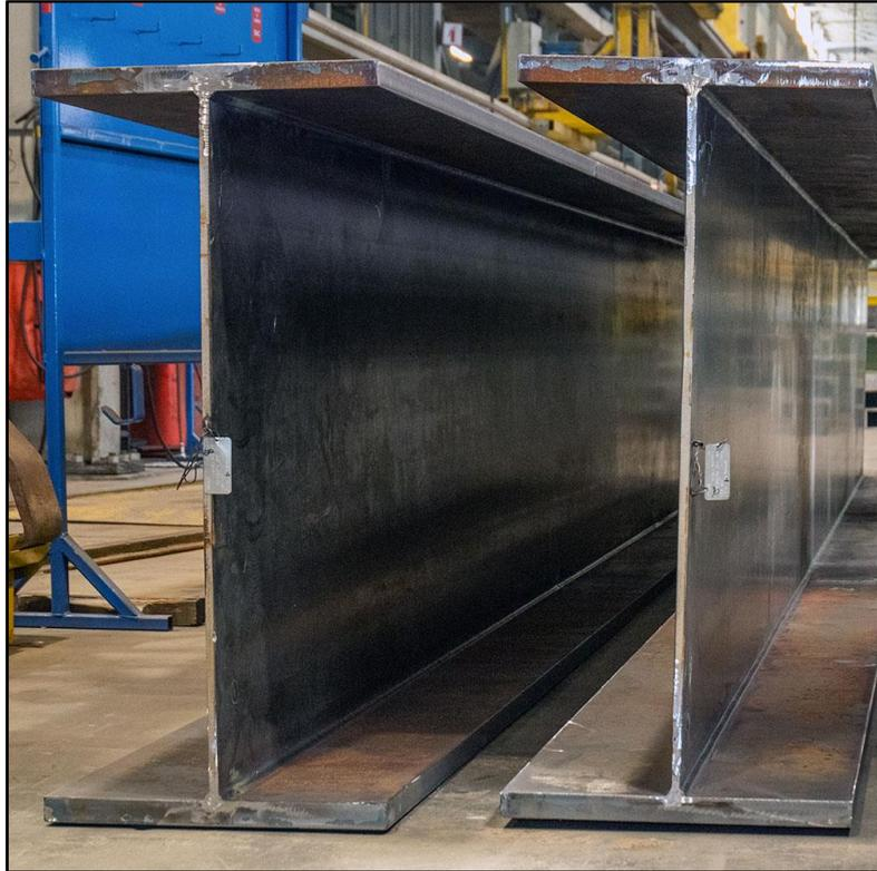
**Figure 1.4.** Welded I-shaped bisymmetric plate girders (Structures, 2021)
