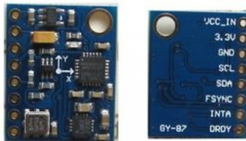
Figure 4.8: Front and back view of the GY-87 IMU board.
