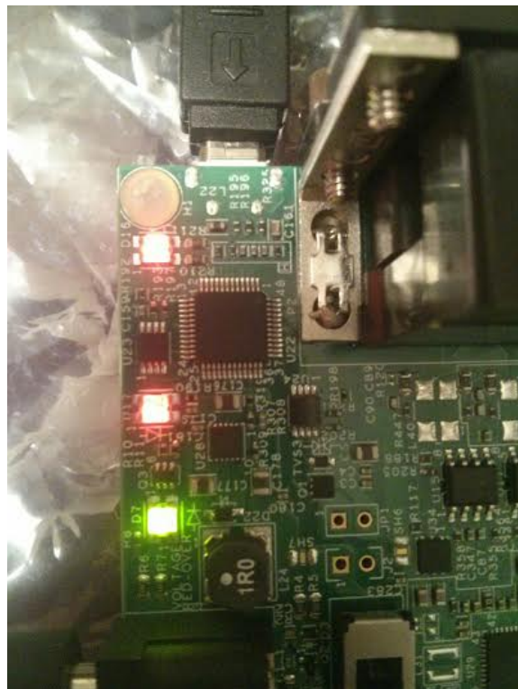
Figure 3.8: Led lights on the board showing that both cores are running.
