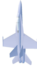
Figure 4.5: Body's position in which gimbal lock occurs.
