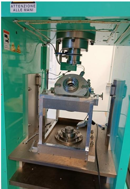
*Figure 2.4. Disassembled pressure vessel.*
