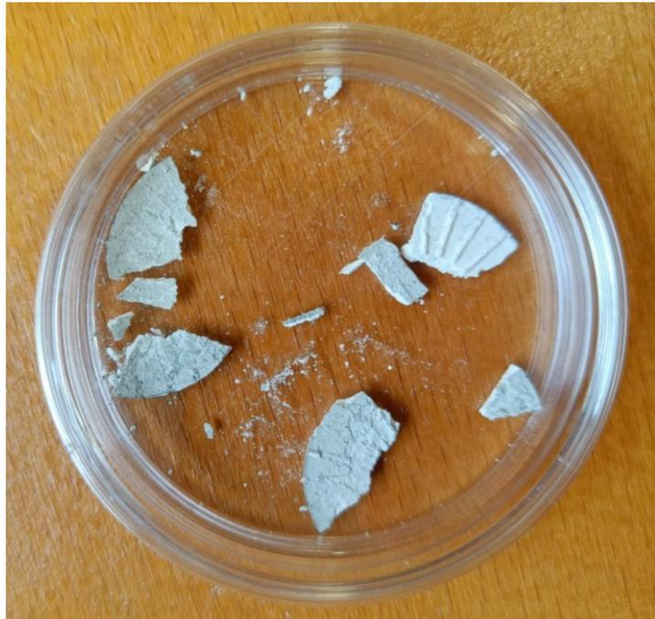
*Figure 2.9. Quartz gouge sample extracted from RoSA.
