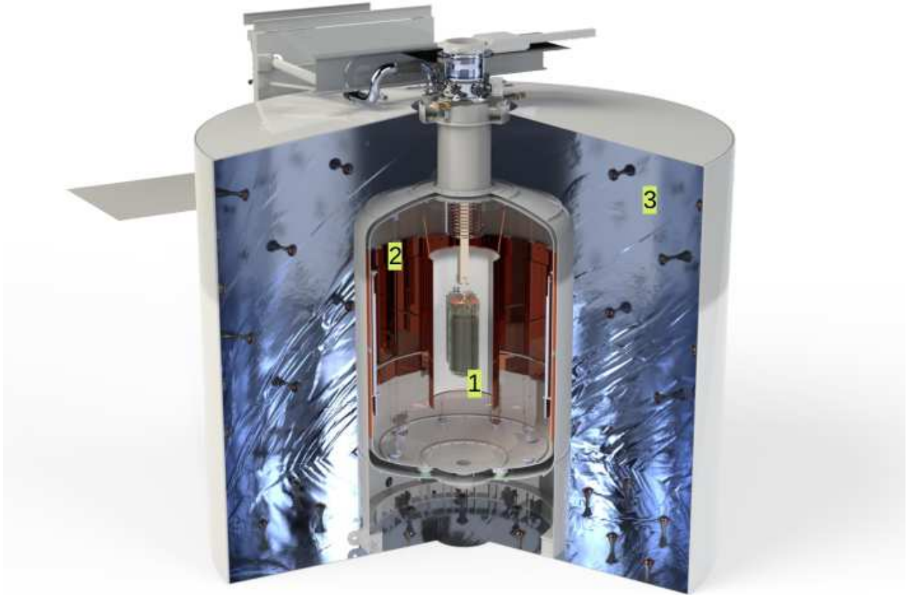
FIGURE 2.1: Sketch of the whole LEGEND experimental setup. From the core: the Germanium detectors strings (1), the cryostat filled with liquid Argon (2) and the water tank (3). Picture credits: Patrick Krause [51].
