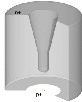
FIGURE 2.4: ICPC detector geometry. Credits: David Hervas Aguilar [51].
