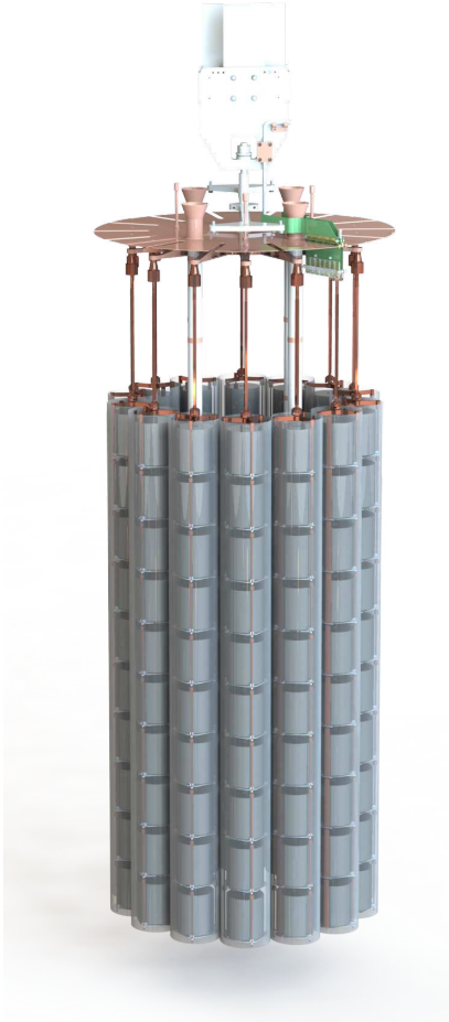
FIGURE 2.2: Sketch of the Germanium detectors array. The nylon mini-shroud wrapping each string is visible in transparency. Credits: Patrick Krause [51].
