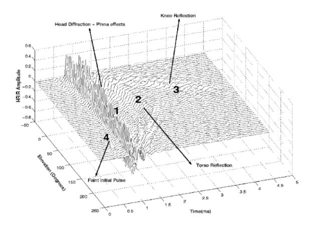
**Figure 1.14:** The HRIR shown as a mesh plot for the right ear for subject 10 in the CIPIC database for azimuth angle  $\theta = 0^{\circ}$  for all elevations varying from  $-45^{\circ}$  to  $+230.625^{\circ}$ . The faint initial pulse, the torso reflection, and the knee reflection can be clearly seen in this plot. Original plot from [19].
