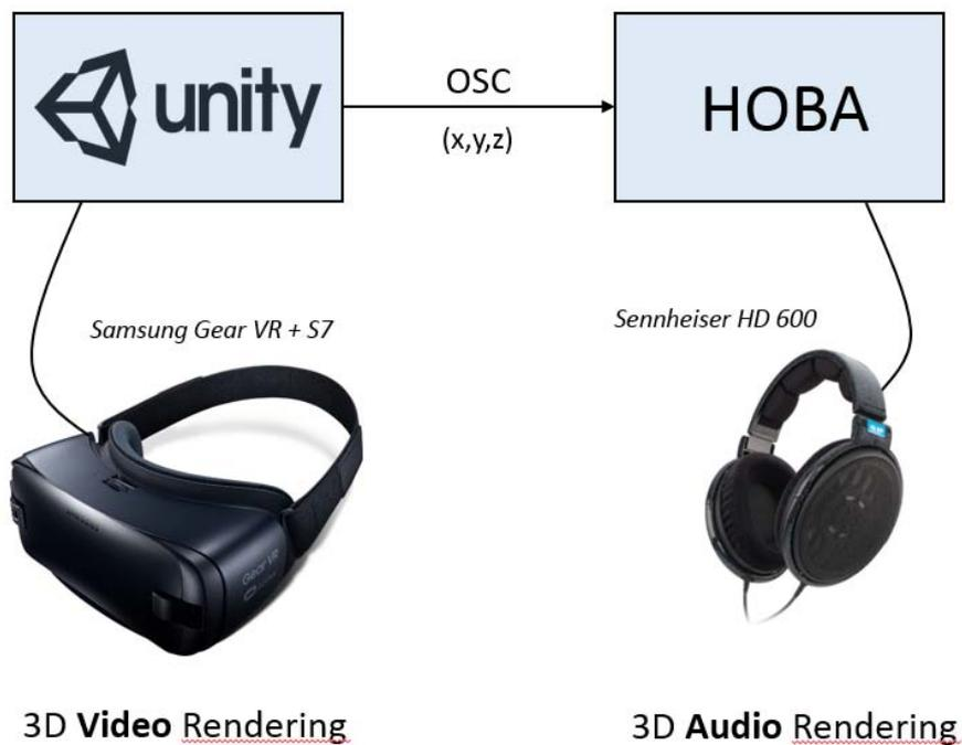
**Figure 3.1:** Block scheme of application tools.
