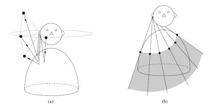
Figure 1.8: Effects of torso and shoulders: (a) reflections (b) shadowing
