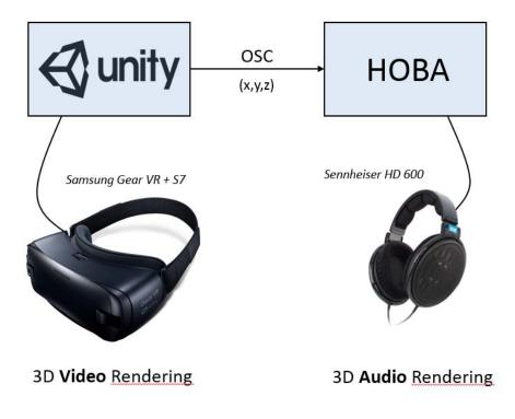
Figure 3.1: Block scheme of application tools.
