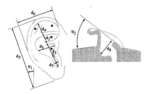
Figure 1.13: CIPIC database pinna measurements. Original picture from [1].
