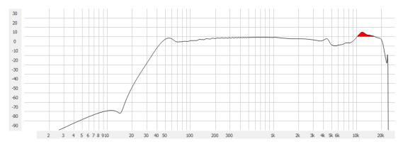
Figure 3.4: Sennheiser HD600 HpTF loaded in the APO Equalizer.
