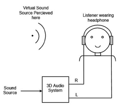
Figure 1.4: Virtual Auditory Display: binaural synthesis. Original picture from [5].
