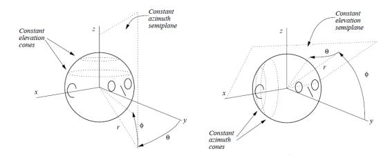
Figure 1.9: (a) Vertical-polar coordinate system (b) interaural-polar coordinate system.
