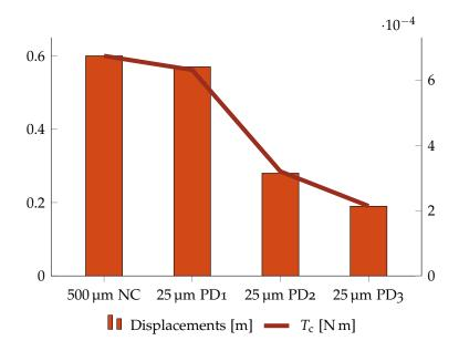
Figure 5.1: Comparison between the displacements and the torques needed to control the satellite in the stiffened case with 500 µm thick panels and three entirely controlled systems in low LEO with inertial attitude.
