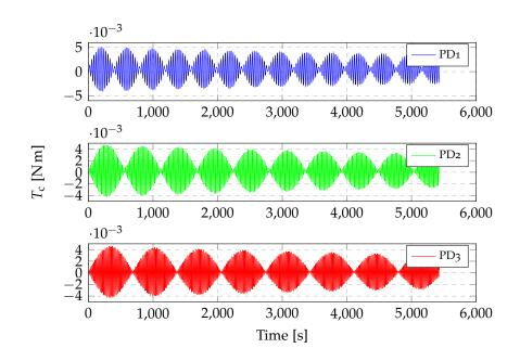
Figure 4.13: Control torques on the satellite at 300 km altitude with nadir pointing attitude (see table 4.3).
