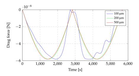
Figure 2.7: Drag force at 500 km for panels of different thicknesses.
