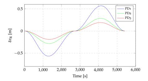
**Figure 4.3:** Displacements of the right tip at 300 km altitude with inertial attitude with controlled systems (see table 4.2).
