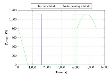
**Figure 2.5:** Instantaneous power production of the two simulated 500 µm thick panels in the two attitude configurations at 300 km height.
