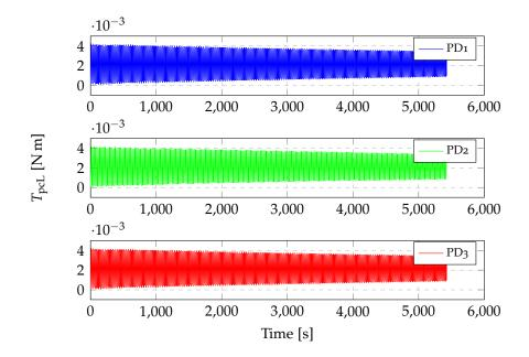
Figure 4.14: Control torques exerted by the control system on the connecting joint between the left panel and the central body (see table 4.3).
