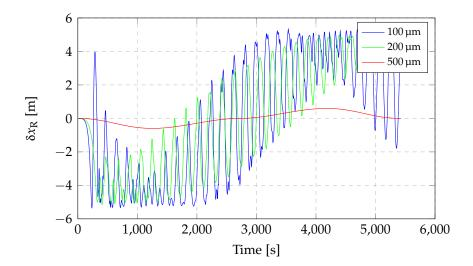
**Figure 3.3:** Displacements of the right tip at 300 km altitude with inertial attitude (see table 3.1).
