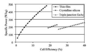
**Figure 1.3:** Specific power of lightweight solar array with thin-film, thin crystalline silicon and crystalline GaAs solar cells as a function of conversion efficiency. [23]
