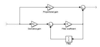
Figure 4.1: PD controller block system.
