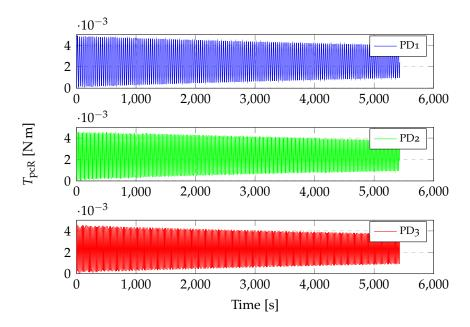
Figure 4.15: Control torques exerted by the control system on the connecting joint between the right panel and the central body (see table 4.3).
