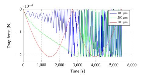
Figure 2.6: Drag force at 300 km for panels of different thicknesses.
