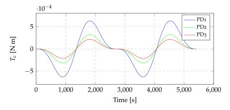
Figure 4.6: Control torques on the satellite at 300 km altitude with inertial attitude (see table 4.2).
