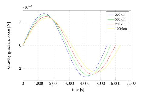
Figure 2.11: X component (along the local vertical) of the gravity gradient force at the tip of a  $500 \,\mu\text{m}$  thick panel at different altitudes.
