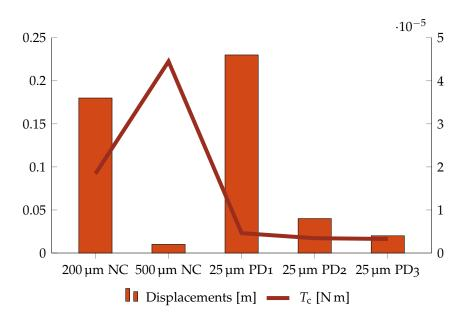
**Figure 5.3:** Comparison between the displacements and the torques needed to control the satellite in the stiffened cases with 200 µm and 500 µm thick panels and three entirely controlled systems in high LEO with inertial attitude.
