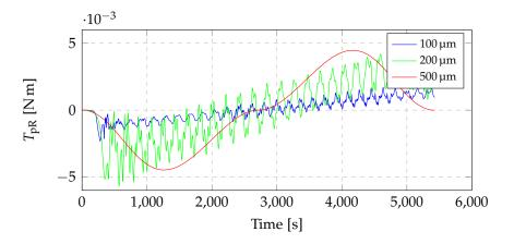
Figure 3.5: Torques transferred from the right panel to the central body at 300 km altitude with inertial attitude (see table 3.1).
