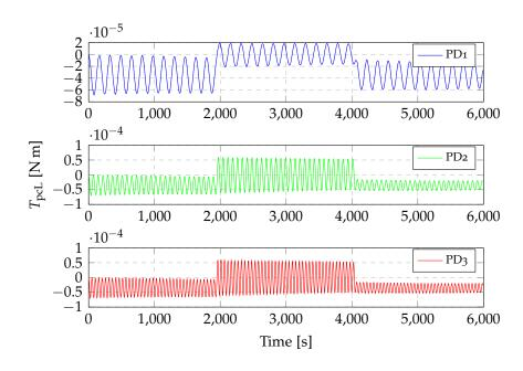
Figure 4.21: Control torques exerted by the control system on the connecting joint between the left panel and the central body (see table 4.5).
