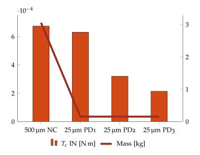
**Figure 5.7:** Comparison between the control torques and the masses of the systems in the stiffened case with 500 µm thick panels and three entirely controlled systems in low LEO with inertial attitude.
