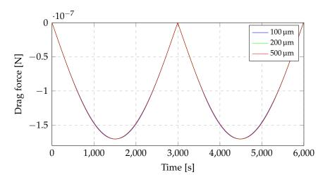
Figure 2.8: Drag force at 750 km for panels of different thicknesses.
