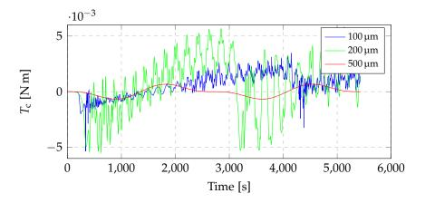
Figure 3.6: Control torques on the satellite at 300 km altitude with inertial attitude (see table 3.1).
