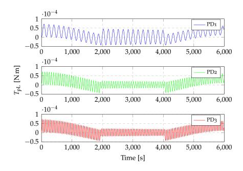
Figure 4.25: Torques transferred from the left panel to the central body at 750 km altitude with nadir pointing attitude (see table 4.6).
