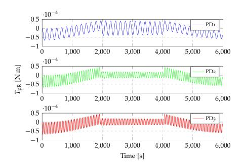
**Figure 4.26**: Torques transferred from the right panel to the central body at 750 km altitude with nadir pointing attitude (see table 4.6).
