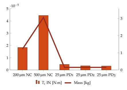
**Figure 5.8:** Comparison between the control torques and the masses of the systems in the stiffened case with 200 µm and 500 µm thick panels and three entirely controlled systems in high LEO with inertial attitude.
