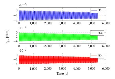
Figure 4.11: Torques transferred from the left panel to the central body at 300 km altitude with nadir pointing attitude (see table 4.3).
