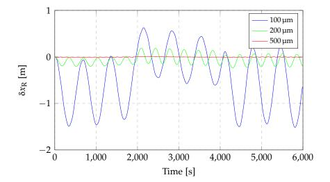
Figure 3.13: Displacements of the right tip at 750 km altitude (see table 3.3).
