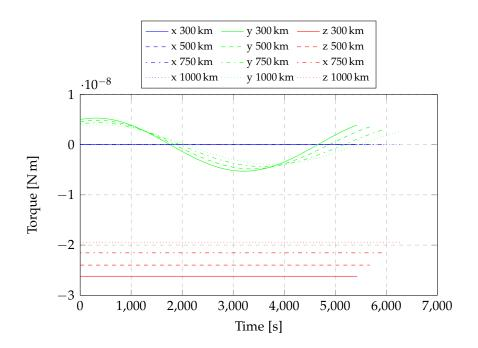
Figure 2.13: Components of the torque due to the interaction of the panels with the magnetic field at different altitudes.
