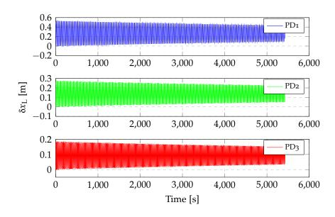
**Figure 4.9:** Displacements of the left tip at 300 km altitude with nadir pointing attitude with controlled systems (see table 4.3).
