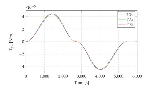
**Figure 4.4:** Torques transferred from the left panel to the central body at 300 km altitude with inertial attitude (see table 4.2).
