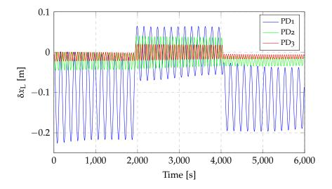
**Figure 4.16:** Displacements of the left tip at 750 km altitude with inertial attitude with controlled systems (see table 4.5).
