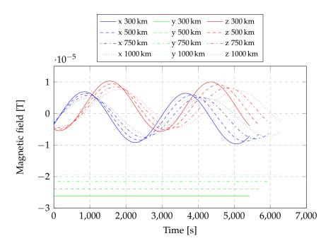
Figure 2.12: Components of the magnetic field at different altitudes.
