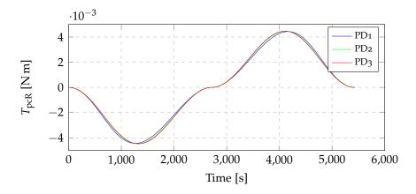
**Figure 4.8:** Control torques exerted by the control system on the connecting joint between the right panel and the central body (see table 4.2).
