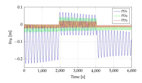
**Figure 4.17:** Displacements of the right tip at 750 km altitude with inertial attitude with controlled systems (see table 4.5).
