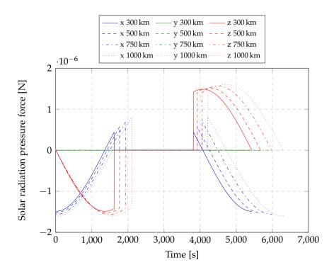
**Figure 2.9:** Force exerted by solar radiation pressure at different altitudes on a 500 µm thick panel in equatorial orbit with inertial attitude, in the *World* CS.
