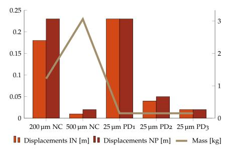
**Figure 5.6:** Comparison between the displacements and the masses of the systems in the stiffened case with 200 µm and 500 µm thick panels and three entirely controlled systems in high LEO.
