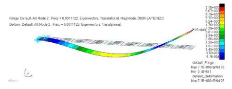
Figure 2.4: Second natural frequency of a 5.51 m long panel.
