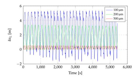
Figure 3.7: Displacements of the left tip at 300 km altitude (see table 3.2).
