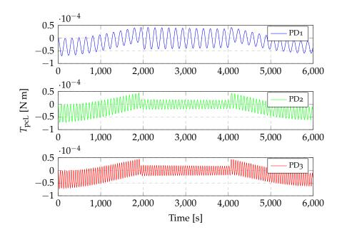
**Figure 4.28:** Control torques exerted by the control system on the connecting joint between the left panel and the central body (see table 4.6).
