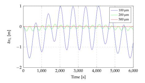
Figure 3.17: Displacements of the left tip at 750 km altitude (see table 3.4).
