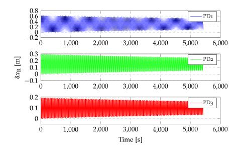
Figure 4.10: Displacements of the right tip at 300 km altitude with nadir pointing attitude with controlled systems (see table 4.3).
