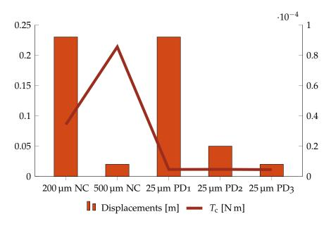
**Figure 5.4**: Comparison between the displacements and the torques needed to control the satellite in the stiffened cases with 200 µm and 500 µm thick panels and three entirely controlled systems in high LEO with nadir pointing attitude.
