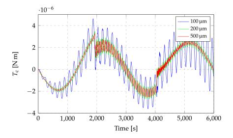
**Figure 4.20:** Control torques on the satellite at 750 km altitude with inertial attitude (see table 4.5).
