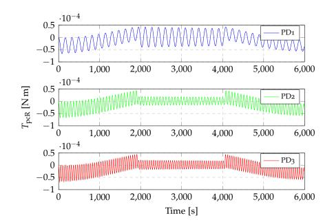
**Figure 4.29:** Control torques exerted by the control system on the connecting joint between the right panel and the central body (see table 4.6).
