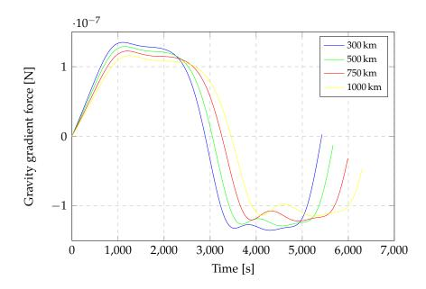
Figure 2.10: X component (along the local vertical) of the gravity gradient force at the tip of a  $25\,\mu m$  thick panel at different altitudes.
