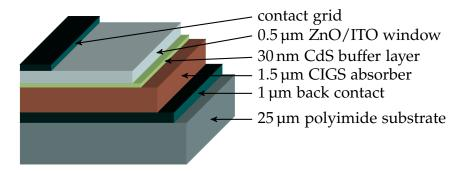
Figure 1.1: Schematic drawing of a flexible CIGS TFSC. Not to scale. [2]
