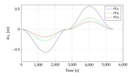
**Figure 4.2:** Displacements of the left tip at 300 km altitude with inertial attitude with controlled systems (see table 4.2).
