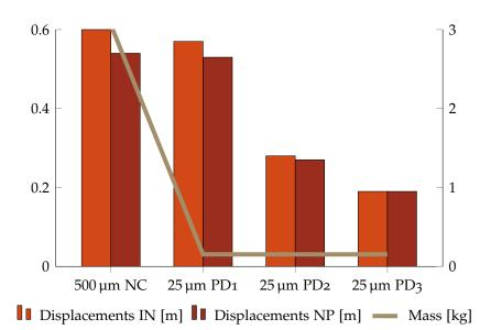
**Figure 5.5:** Comparison between the displacements and the masses of the systems in the stiffened case with 500 µm thick panels and three entirely controlled systems in low LEO.
