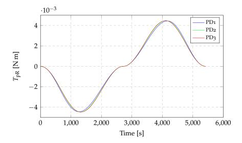
Figure 4.5: Torques transferred from the right panel to the central body at 300 km altitude with inertial attitude (see table 4.2).
