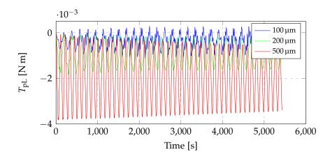
**Figure 3.9:** Torques transferred from the left panel to the central body at 300 km altitude with nadir pointing attitude (see table 3.2).
