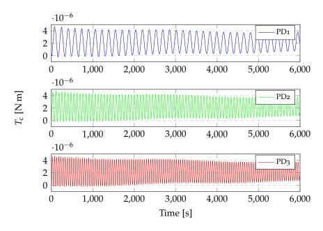
**Figure 4.27:** Control torques on the satellite at 750 km altitude with nadir pointing attitude (see table 4.6).
