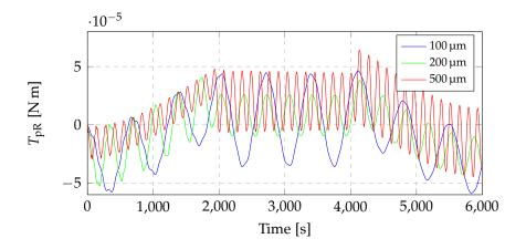
**Figure 3.20:** Torques transferred from the right panel to the central body (see table 3.4).
