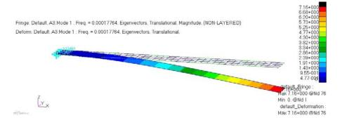
Figure 2.3: First natural frequency of a 5.51 m long panel.
