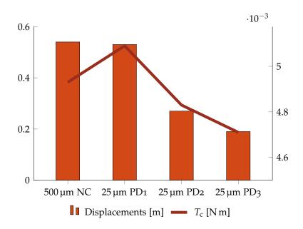
**Figure 5.2:** Comparison between the displacements and the torques needed to control the satellite in the stiffened case with 500 µm thick panels and three entirely controlled systems in low LEO with nadir pointing attitude.
