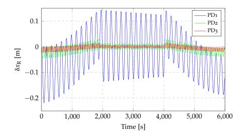
**Figure 4.24**: Displacements of the right tip at 750 km altitude with nadir pointing attitude with controlled systems (see table 4.6).
