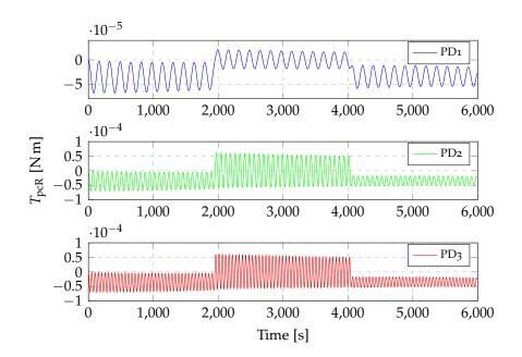
**Figure 4.22:** Control torques exerted by the control system on the connecting joint between the right panel and the central body (see table 4.5).
