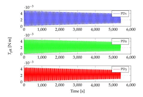
**Figure 4.12:** Torques transferred from the right panel to the central body at 300 km altitude with nadir pointing attitude (see table 4.3).
