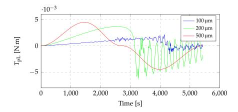
**Figure 3.4**: Torques transferred from the left panel to the central body at 300 km altitude with inertial attitude (see table 3.1).
