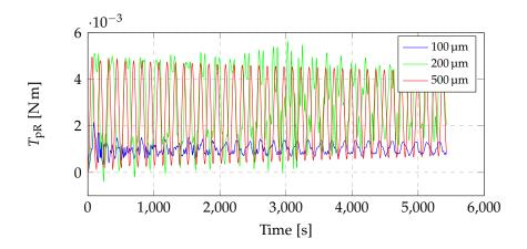
**Figure 3.10**: Torques transferred from the right panel to the central body at 300 km altitude with nadir pointing attitude (see table 3.2).
