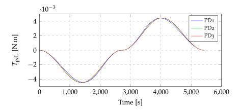
**Figure 4.7**: Control torques exerted by the control system on the connecting joint between the left panel and the central body (see table 4.2).
