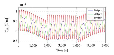
**Figure 3.19:** Torques transferred from the left panel to the central body (see table 3.4).
