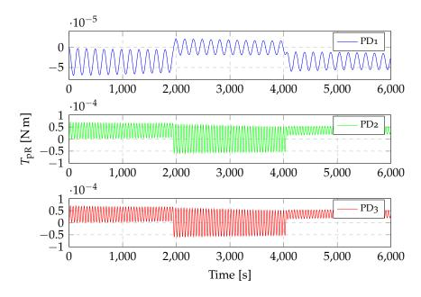
Figure 4.19: Torques transferred from the right panel to the central body at 750 km altitude with inertial attitude (see table 4.5).
