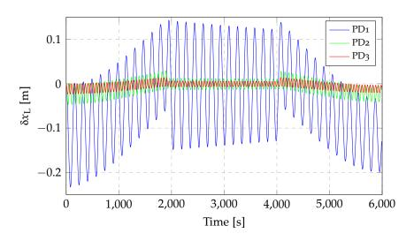
Figure 4.23: Displacements of the left tip at 750 km altitude with nadir pointing attitude with controlled systems (see table 4.6).
