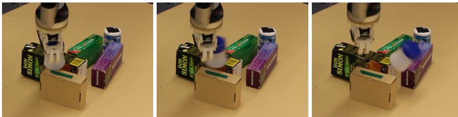
Fig. 7.3: Unstable grasp that makes the object slip out.
