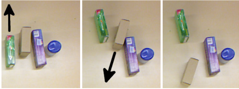
Fig. 7.2: Unexpected outcome of the pushing action. In the first scene the robot had to push the green box away but it accidentally moved also the brown box. The green box was not graspable after being pushed, the robot replanned and decided to move the brown one.
