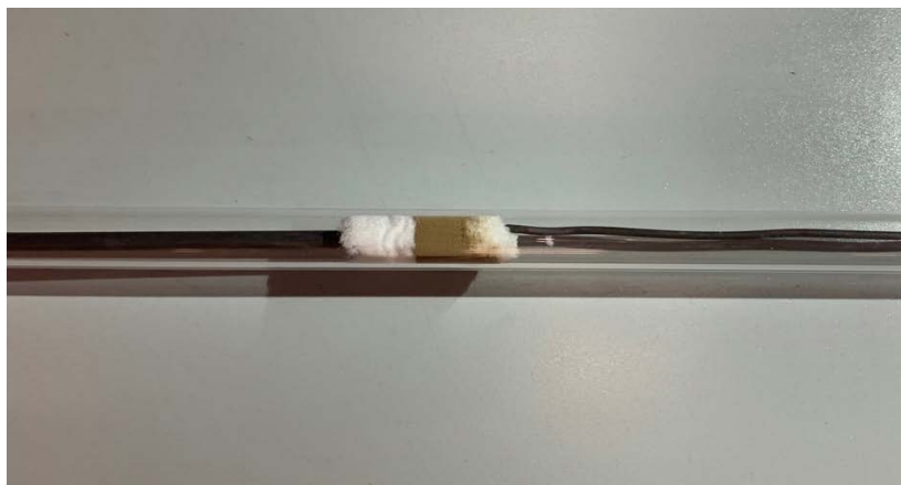
Figure 3.3: Catalytic bed held in place by quartz wool
