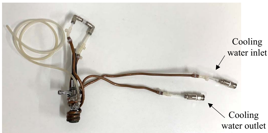
Figure 2.4: Cooling system of the atomiser
