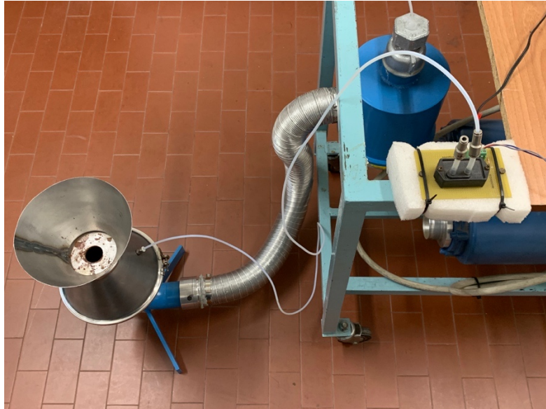
Figure 2.12: Pressure transducer connected to the filter pack
