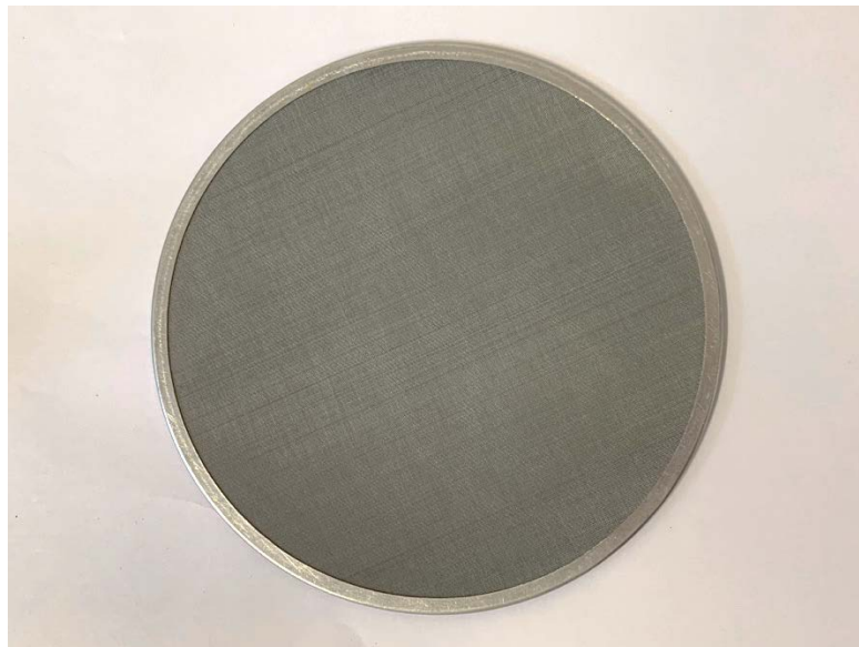
Figure 2.23: Filter utilised in the new experimental set-up
