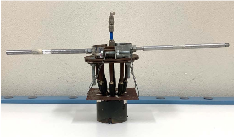
Figure 2.6: Burner with its additional structure
