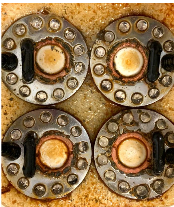
Figure 4.1: Deposition of metal precursors on the atomisers
