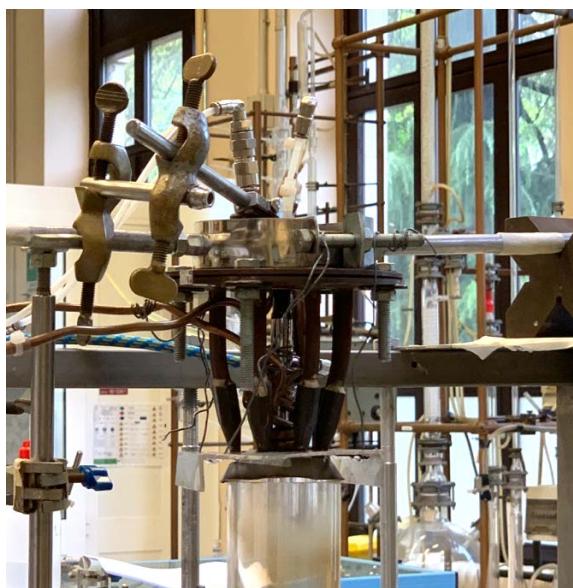
Figure 2.14: New burner structure realised to adapt it to the quartz tube
