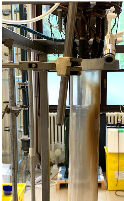
Figure 2.16: Catalyst depositing unevenly on the walls of the quartz tube
