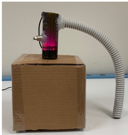
Figure 2.18: New feeding system with one atomiser
