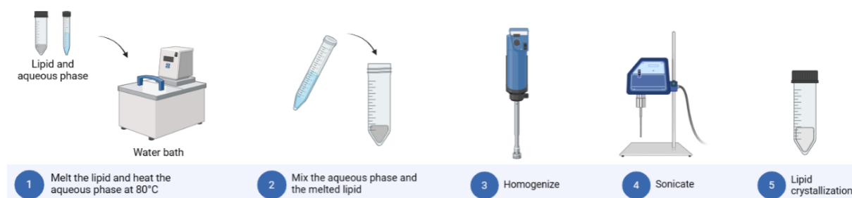
Figure 3.7: Schematic representation of the steps to prepare solid lipid nanoparticles
