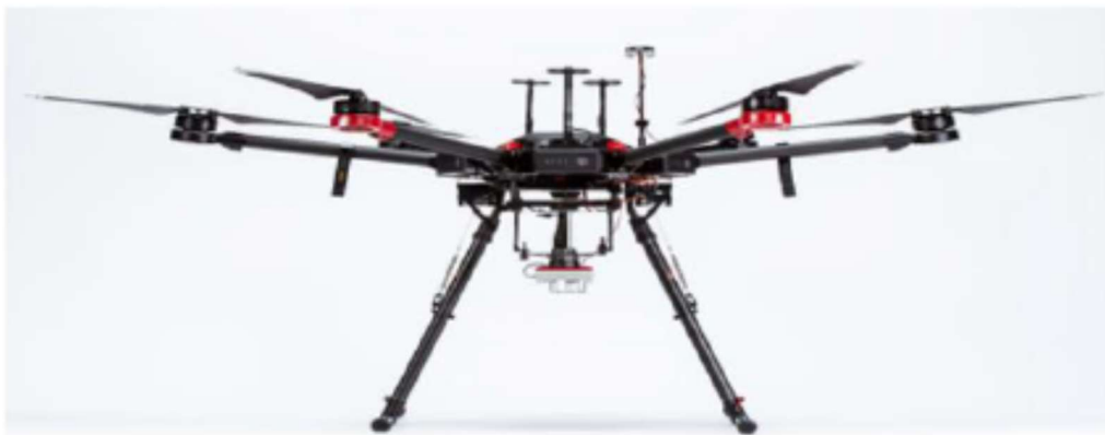
Figure 13 The DJI Matrice 600 drone used in aerial monitoring activities.
