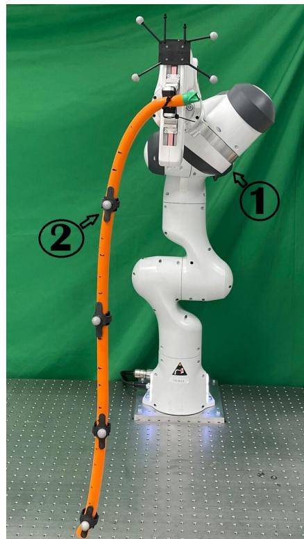
(b) 1. shows the Franka Panda robot; 2. shows the DLO considered
