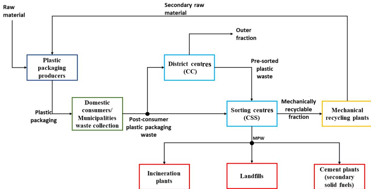
*Figure 1.3: Block Flow Diagram of the Italian traditional packaging waste supply chain*
