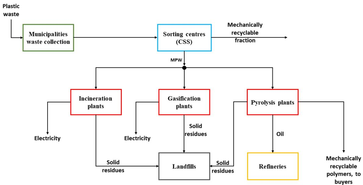
*Figure 1.4: Block Flow Diagram of the Italian alternative packaging waste supply chain*
