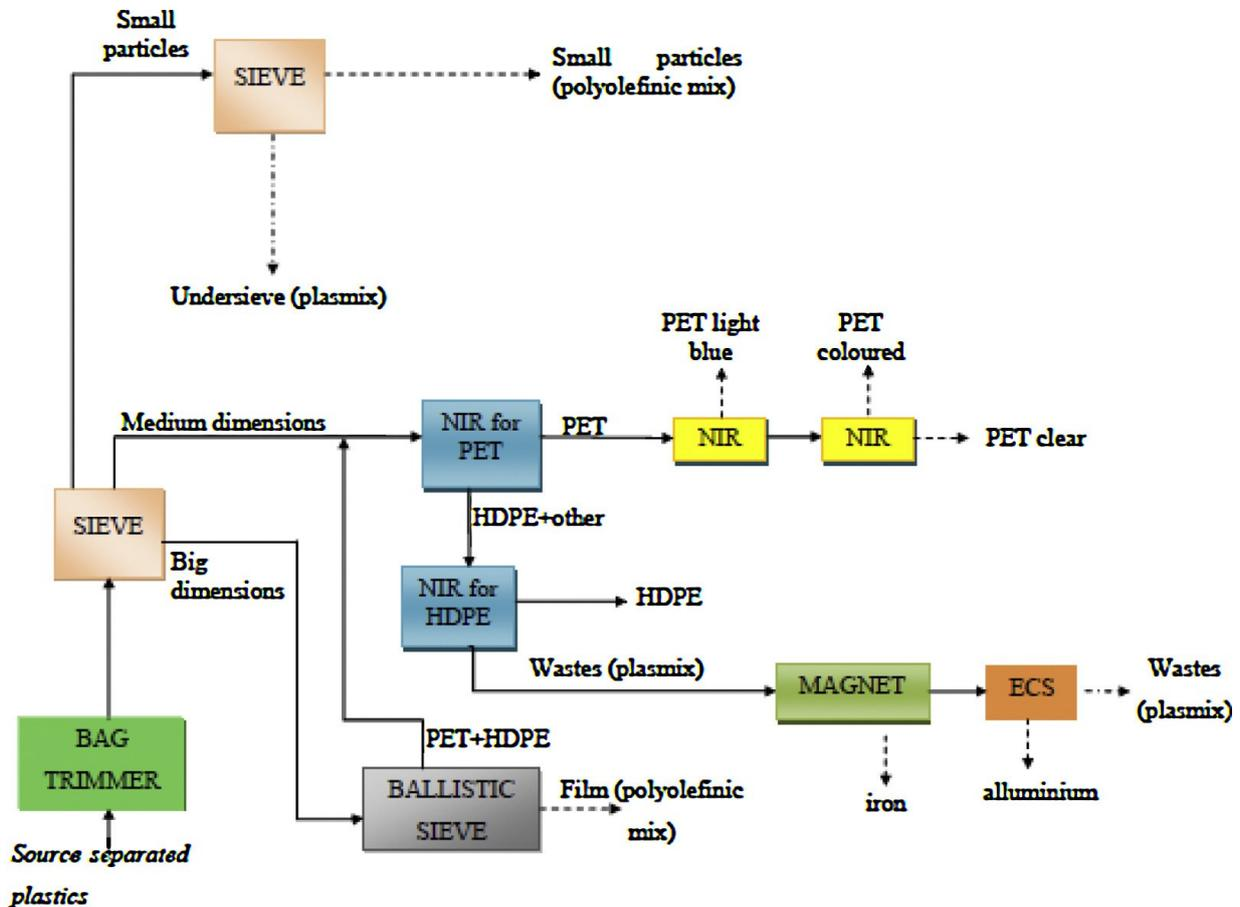
Figure 2.4: Scheme of a sorting centre functional units (Rigamonti et al., 2013)
