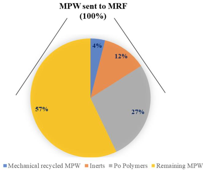
**Figure 2.2:** Material balances for a MRF in a PO\_Pyrolysis plants
