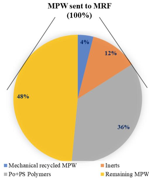
**Figure 2.3:** Material balances for a MRF in a PO\_PS\_Pyrolysis plant
