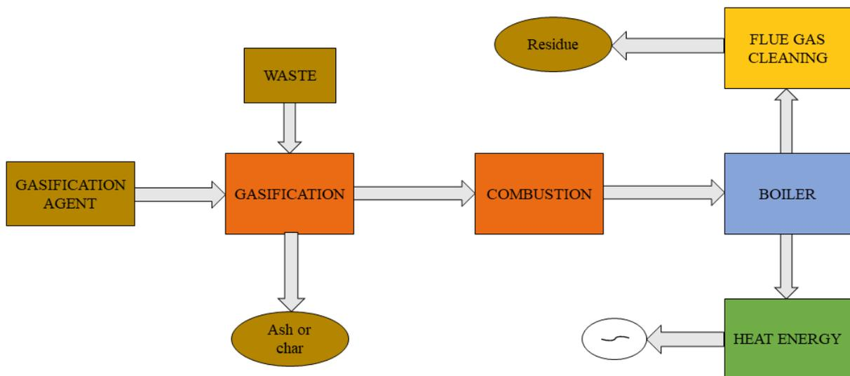
**Figure 1.6:** Simplified scheme of a gasification plant for electricity production (Arena et al., 2011)
