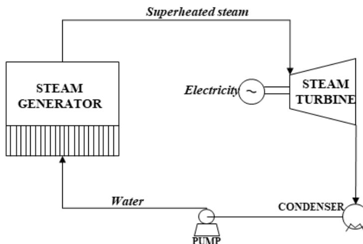
**Figure 1.5:** Simplified scheme for electrical production from an incineration plant (Lombardi et al., 2014)
