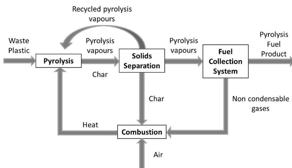
**Figure 1.7:** Simplified scheme of a pyrolysis unit (Fivga and Dimitriou, 2018)
