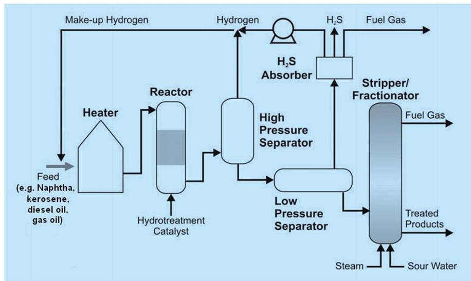
*Figure 2.6: Typical HDS unit in an oil refinery*
