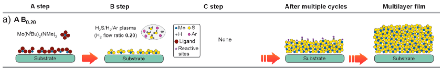
Figure 1.15: Schematics of an atomic layer deposition process (ALD) [Mattinen et al., 2023].
