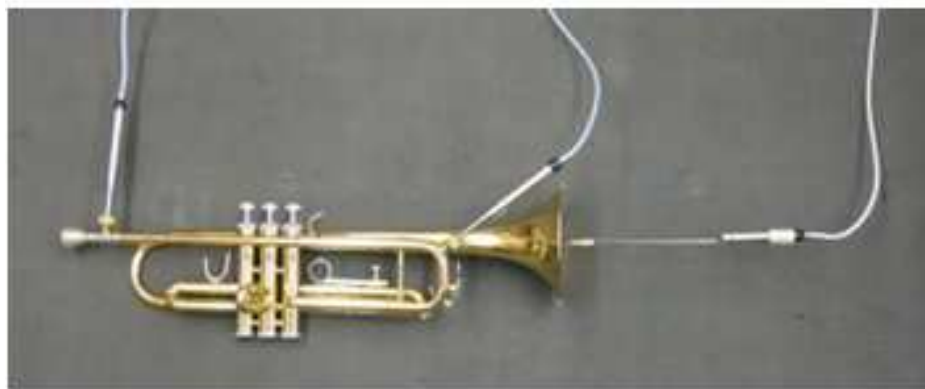
Figure 2.5: Microphone placement on the trumpet[18].
