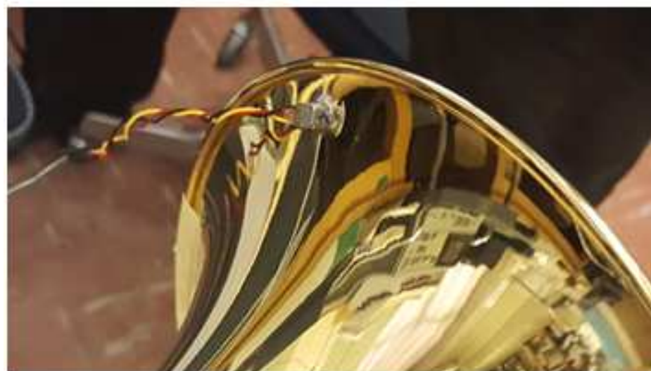
Figure 2.6: Accelerometer placement on the bell of the trumpet[18]
