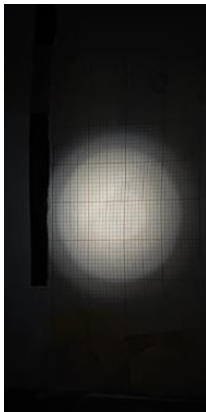
Figure 16: The diameter of the 8 mm focal lens at 50 cm over graph paper. It is possible to see how big the divergence is.
