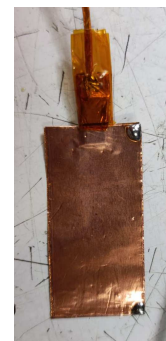
Figure 5: The probe tip sealed with insulated connector to the Kap4 cable.
