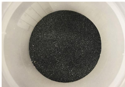
Figure 4.43: Appearance of the diluted bed after the two TPR-TPO series.
