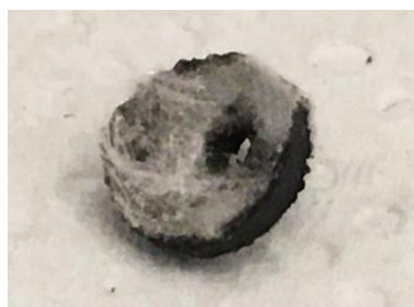
Figure 4.5: Spent CuO bed after 11 redox cycles.
