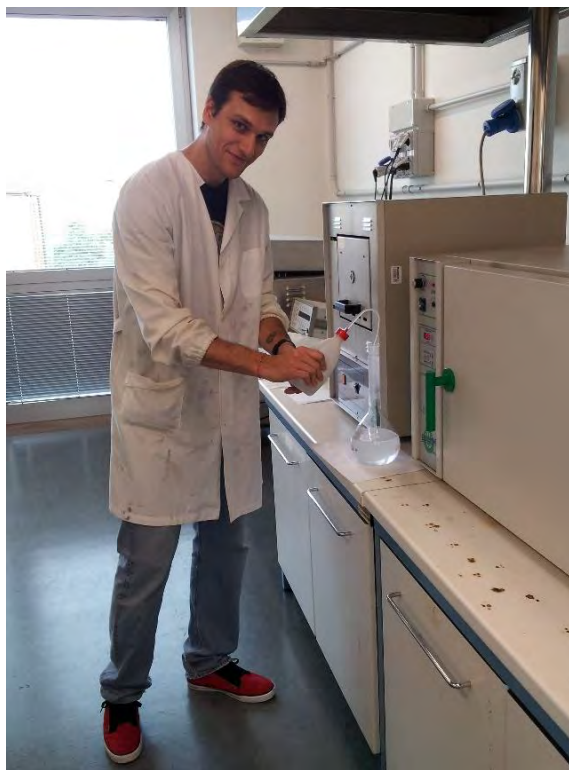
Figure 3. Me diluting to the mark the sodium hydroxide solution for pH control
