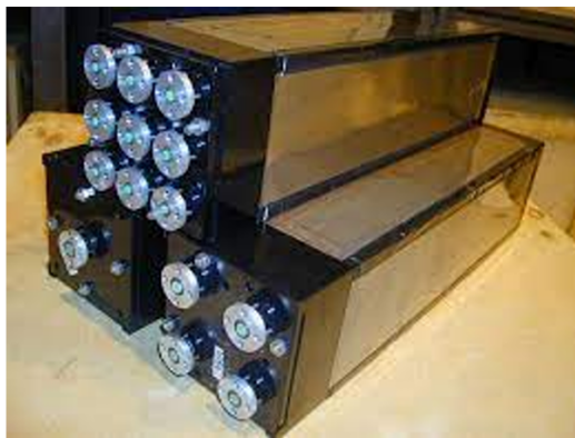
Figure 2.6: The ECAL modules with Shashlik technology with 9, 4, 1 cell per module (left). The schematization of a 9-cell Shashlik module structure (right).
