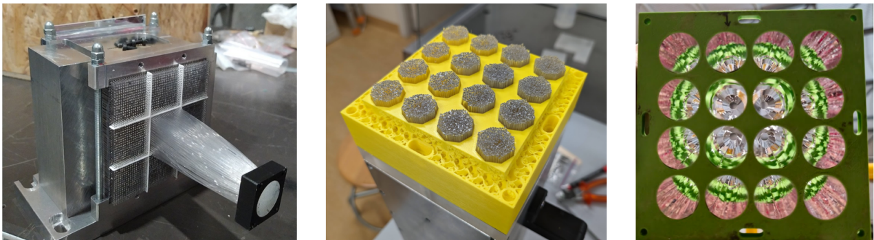
Figure 5.4: Picture Pb/Poly prototypes while being assembled. The back side of a prototype with visible fibers is separated into 9 cells and grouped with a bundle (left). The back side of the actual test-beam prototype with 16 cells already grouped in bundles (middle). Front view of a light guide (right).
