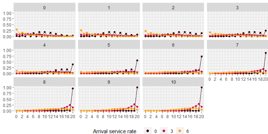
Figure 5.6: Example of \mathbf{P} matrix estimate for arrival queues. Separately for the number of aircraft waiting to be served at the beginning of the period, each plot shows the state probability of the airport system with regards to the number of stages of work to be completed at the end of the time period, which is t = 16 (13.00–13.30).
