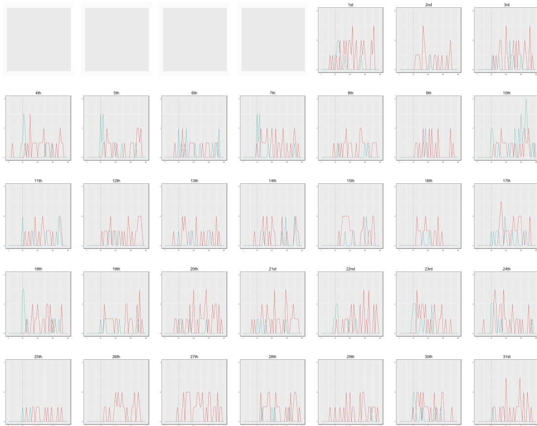
Figure 5.5: Distribution of the observed arrival and departure queues lengths for December 2017. Arrivals are marked with the red line, departures with the blue. Representation is detailed for each day of the month, with reference to each 30-minute length time interval. The dotted vertical line is in correspondence to the time period t = 1 , i.e. between 5.30 a.m. and 6.00 a.m.
