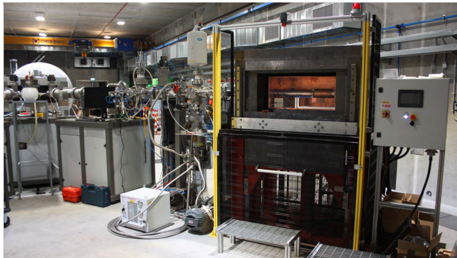
FIGURE 2.3: March 2025 image of the beamline into the open interaction chamber. Visible is a prototype of the NaI scintillator and cryocooling for the cold trap.
