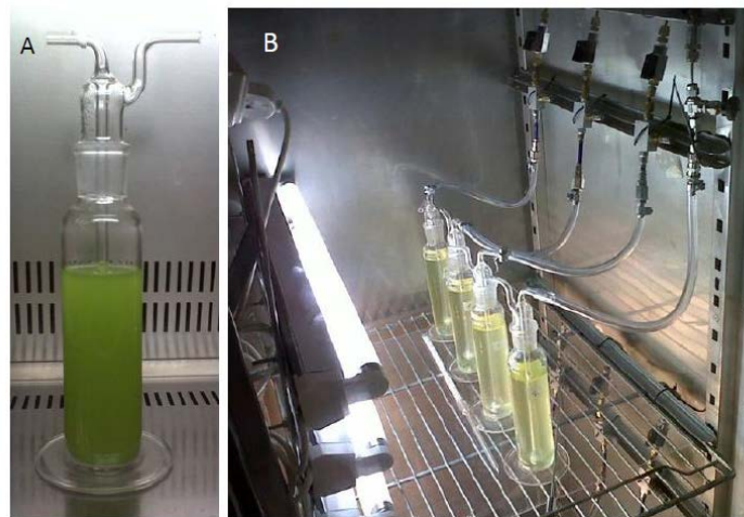
Figure 2.1 A) Drechsel bottle B) Bottles connected to the feed of \text{CO}_2 -enriched air.
