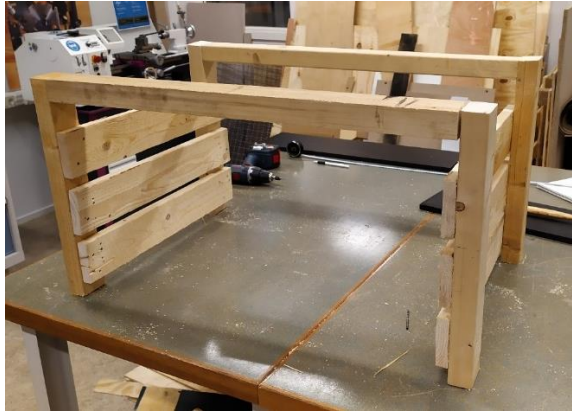
Fig. 12 - Work in progress of building the small scale 3-levels rack.
