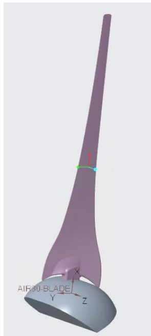
Figure 4-16 Air 30 blade coupled with hub
