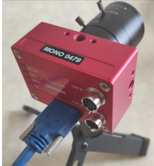
Figure 3.6: The DAVIS346 event-camera used in this work [14].
