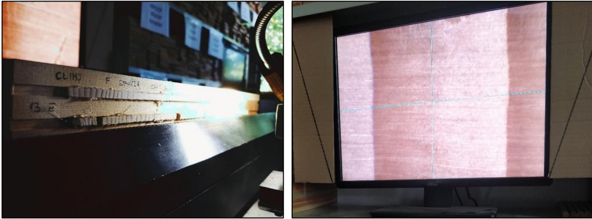
Figure 8 – 9: Cores measuring by Biritz GmbH with accuracy of 0.01 mm. Annual rings are considered reliable until their inclination does not exceed 70°, represented by the black lines outside the screen.
