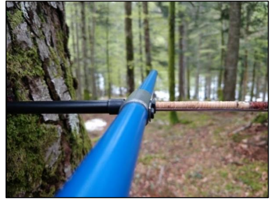
Figure 5 – 6: silver fir - Northern and Eastern cores extraction with Pressler increment borer in Cansiglio_01 study plot.
