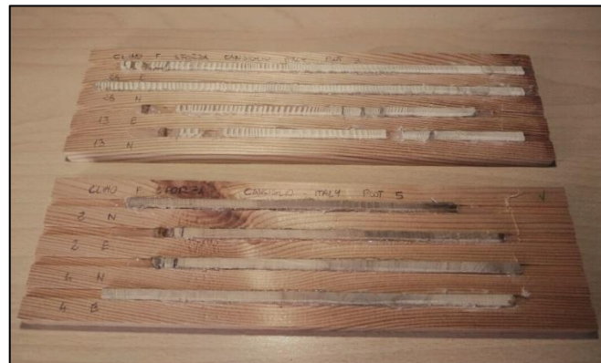
Figure 7: woody core samples glued on the prefabricated support. The samples come from the Cansiglio_01 study plot: it is possible to appreciate the difference in rings clearness between the silver fir (top support) and European beech (bottom support).
