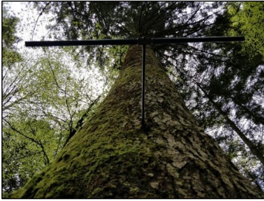
Figure 5 – 6: silver fir - Northern and Eastern cores extraction with Pressler increment borer in Cansiglio_01 study plot.
