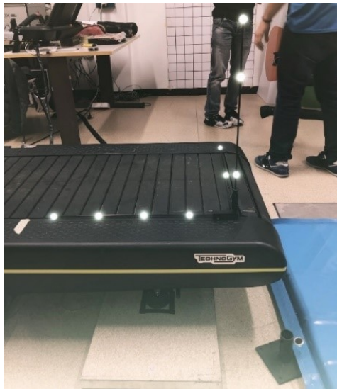
Figure 3.4. Calibration of the system with global reference triad
