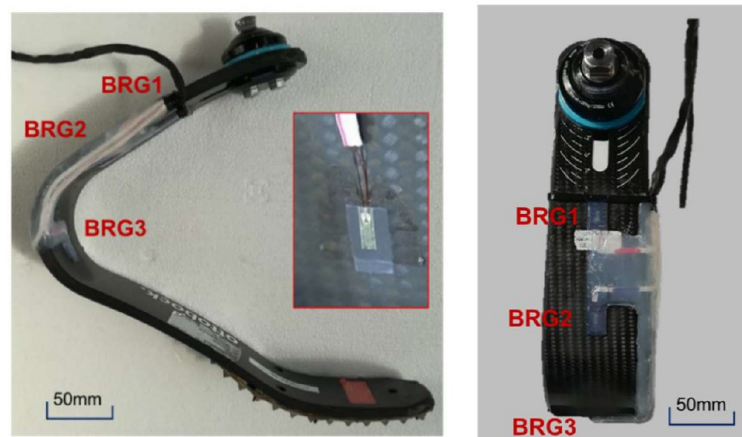
Figure 2.10. Instrumented RPF: strain gauge bridges applied to a Ottobock Runner Cat. 4 RPF [Petrone et al., 2020 [44]]
