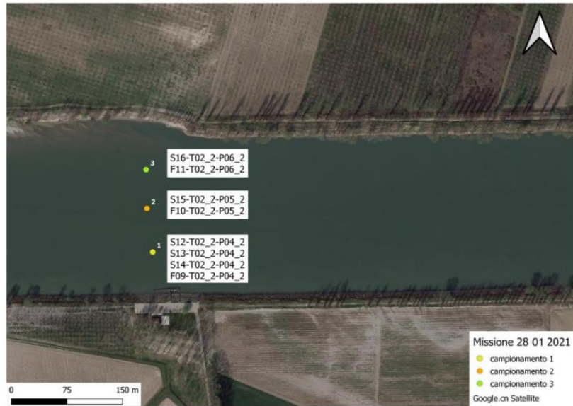
Figure 13 - Sampling points of solid transport at the bottom and in suspension located between nodes 33 and 34. Source: Schippa, 2021.
