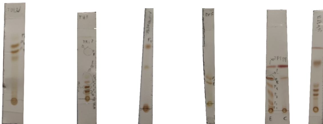
3. from left to right, TLCs of the various reactions using different solvents: toluene, THF, acetonitrile, DMF, ethanol, chloroform and ethanol (specific)
