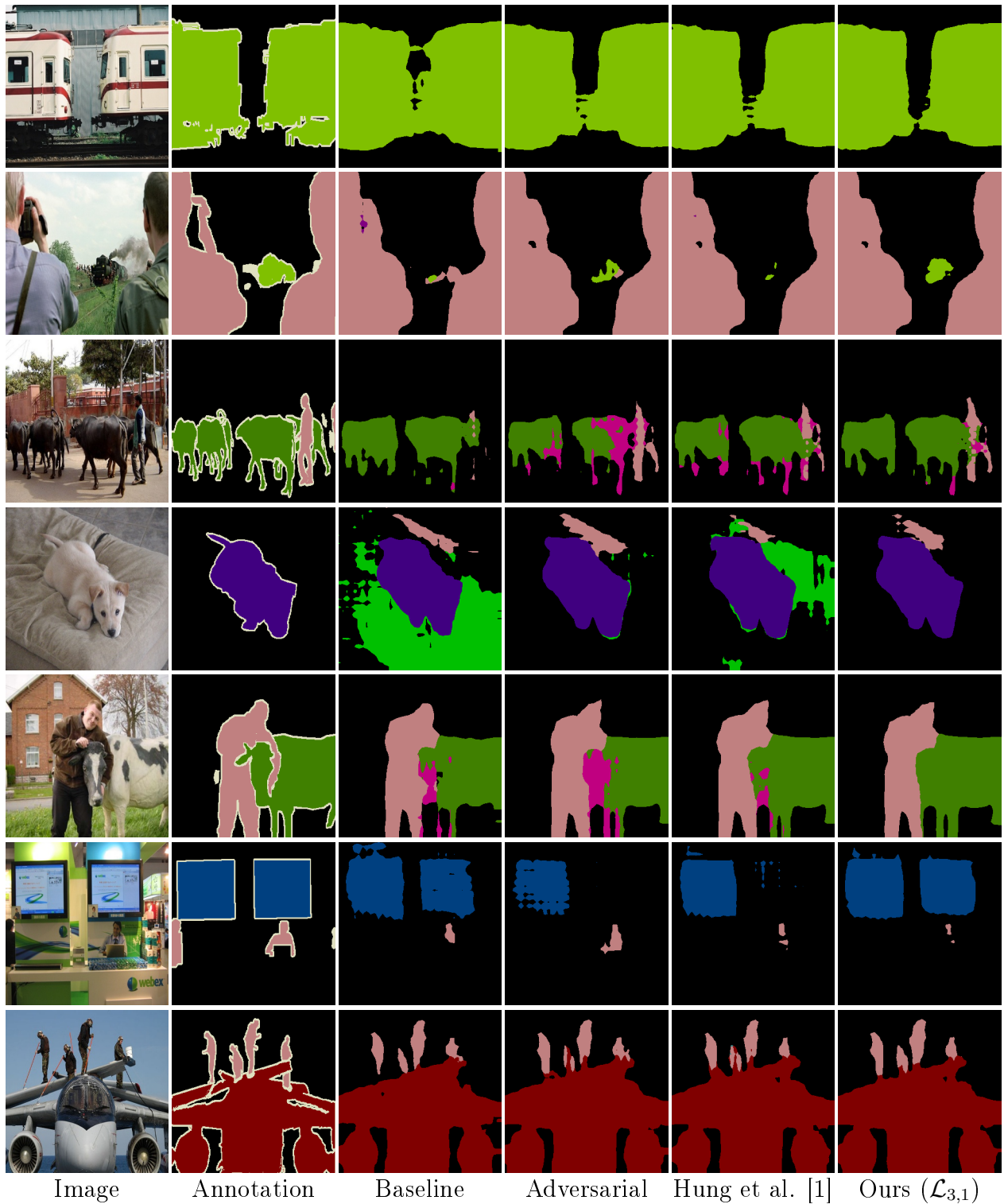
FIGURE 7.2: Extra examples of correct semantic segmentation of some sample scenes extracted from the PASCAL VOC2012 validation dataset. The network is trained using half of the dataset as annotated data and the remaining as unsupervised data
