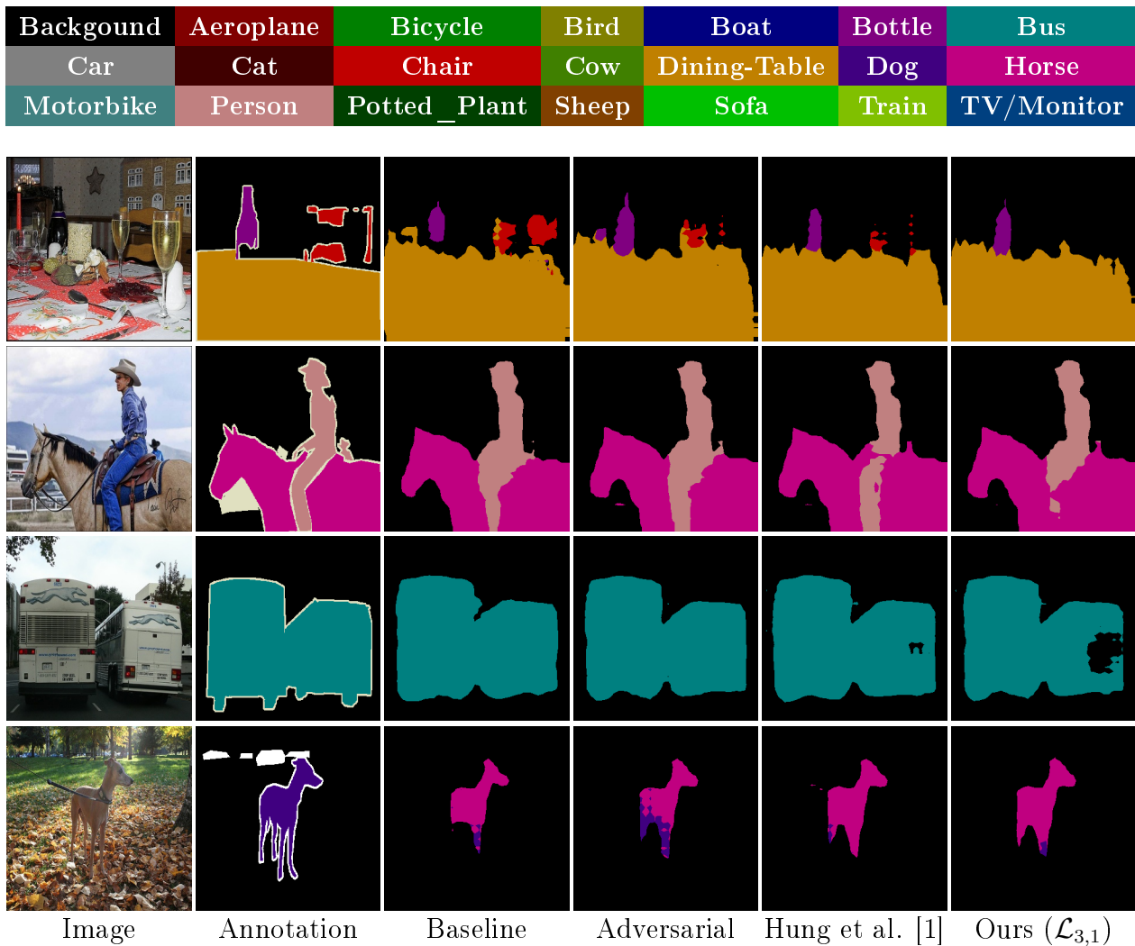
FIGURE 7.1: Extra examples of incorrect semantic segmentation of some sample scenes extracted from the PASCAL VOC2012 validation dataset. The network is trained using half of the dataset as annotated data and the remaining as unsupervised data
