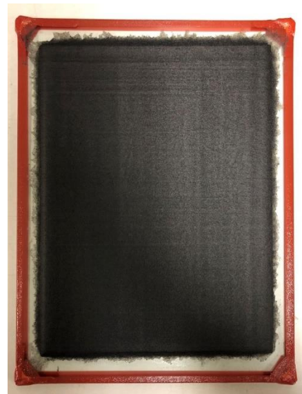
FIG. 8.20 Laminato [0_2/90_4]_s post-autoclave.
