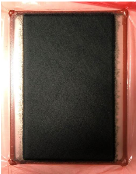
FIG. 8.19 Laminato [+60_3/-60_3]_s post-autoclave.
