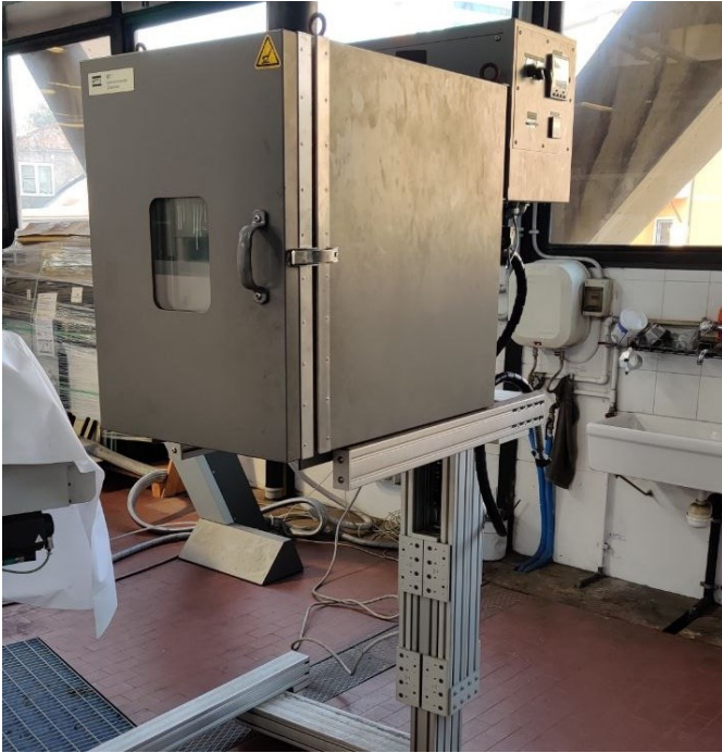
Figure 2.2.1: Climate Chamber disconnected from the MTS-322
