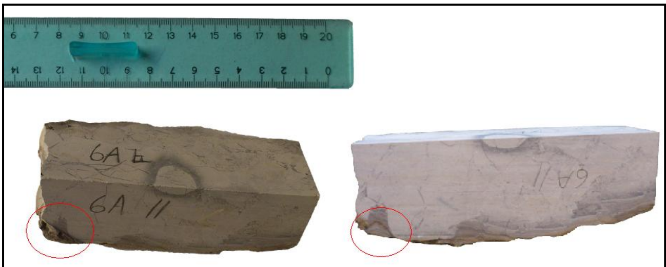
Figure 5.16 Sample 6A before (on the left) and after (on the right) the operations of pre-polishing: the imperfection presents on the left is removed
