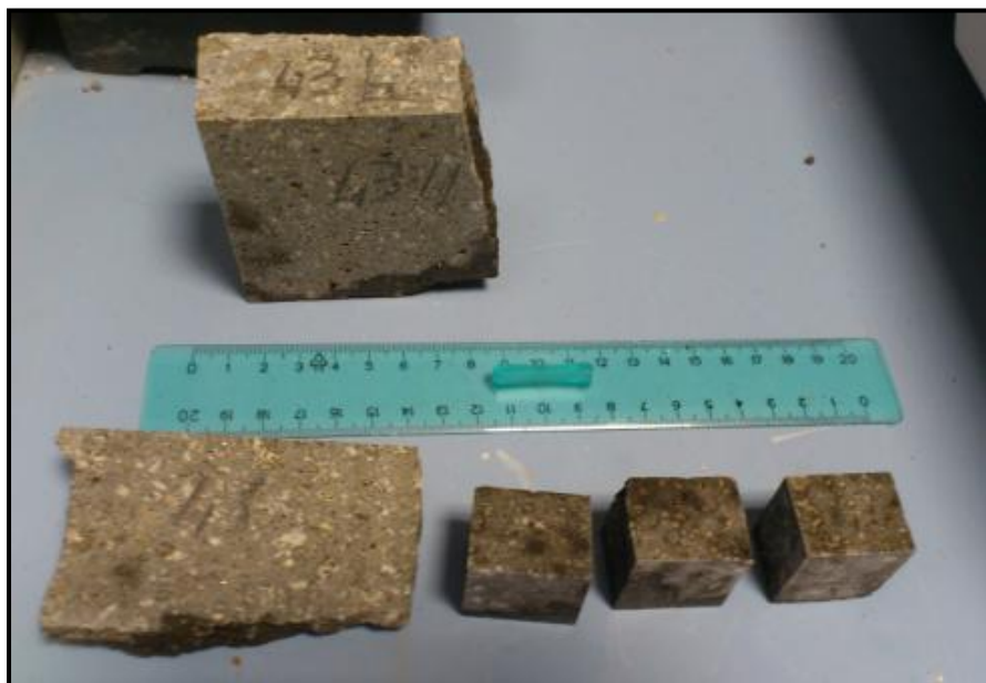
Figure 5.6 Results of Cutting operations for the sample number 43 with the miter saw "Unitom 2"
