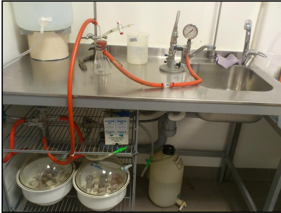
Figure 5.8 Near-vacuum conditions are maintained for 24 hours for both dryers, both connected to the vacuum pump through the orange tubes.
