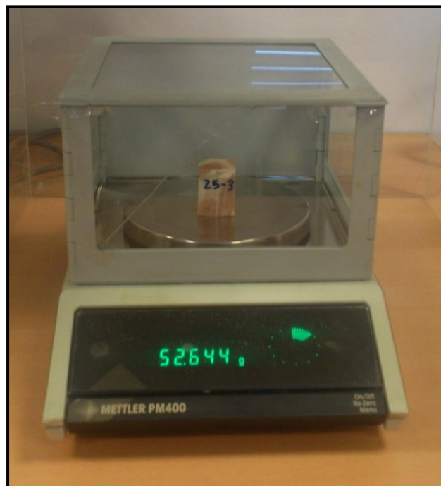
Figure 5.12 Cube number 25-3 in positioned above the balance for the measure of saturated sample in air (ms)
