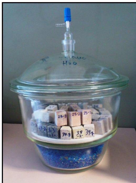
Figure 5.7 Dryer containing cubes removed from the oven
