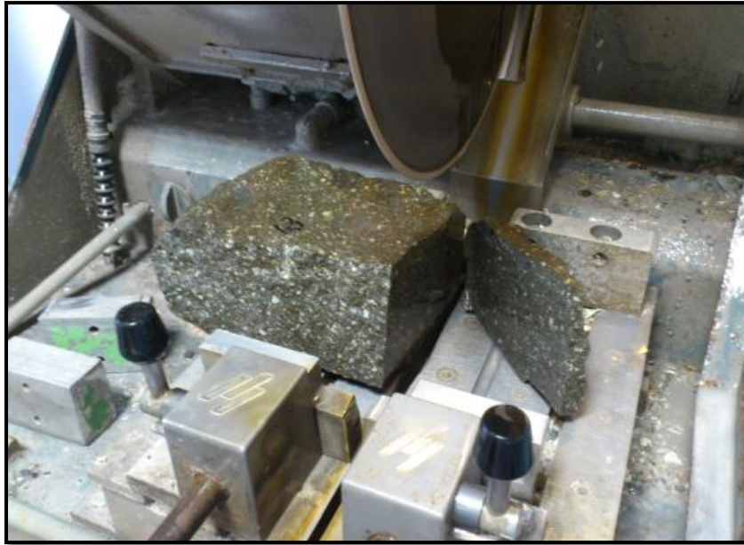
Figure 5.5 Cutting operations for the sample number 43 with the miter saw "Unitom 2"
