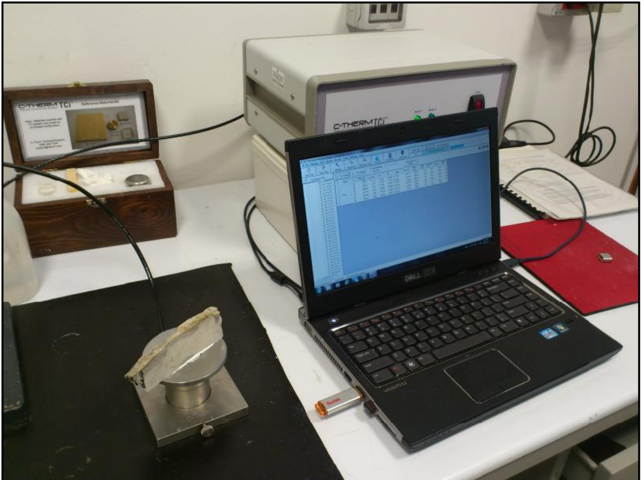
Figure 5.18 Measurement of the thermal properties on the sample 6A
