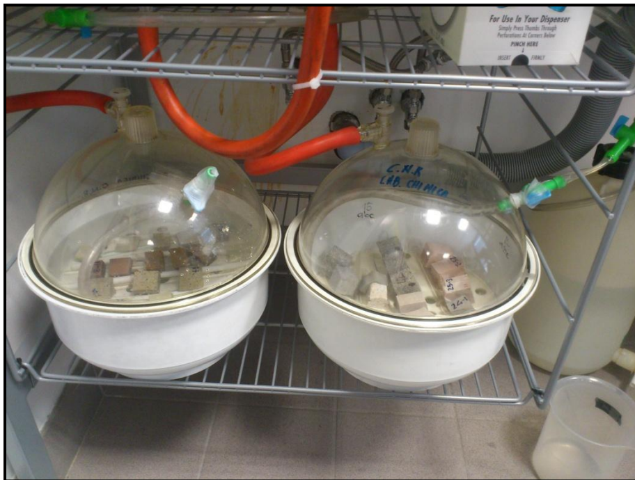
Figure 5.9 The filling of the dryers with demineralized water: the dryer in the left is already filled while the right one is in the filling phase. The water is introduced into the opening through the transparent small tube and adjusted by the green and blue tap.
