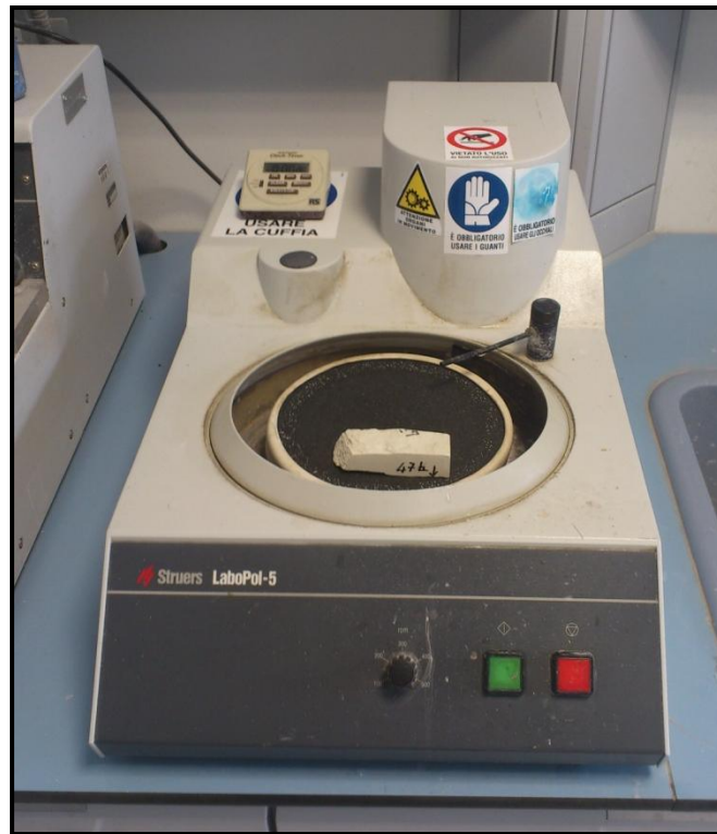
Figure 5.15 Sample 47 after the operation of pre-polishing
