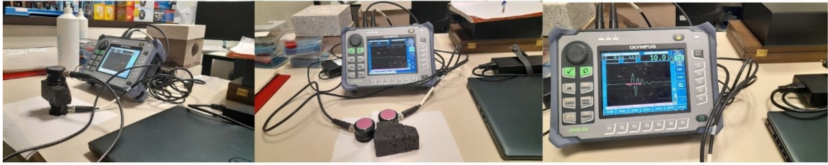
Fig 4.10: Elastic wave propagation time measurement with Epoch 600.
