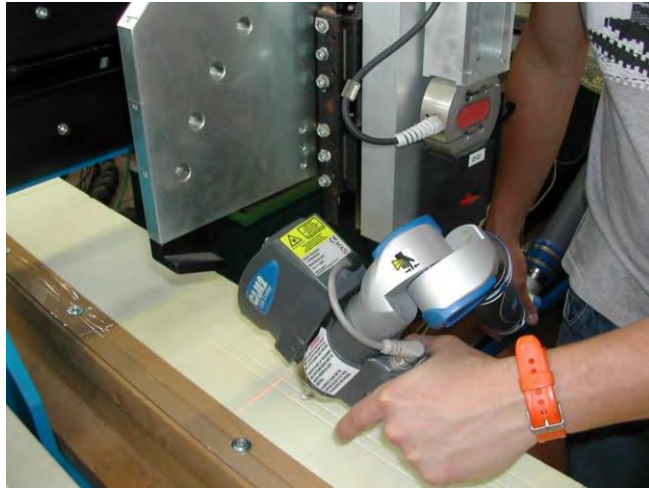
Figure 5.12 Laser scan with Faro ScanArm
