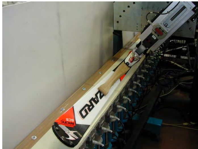
Figure 5.11 Ski characterization with Slytech bench and innovative approach of foam snow mimic
