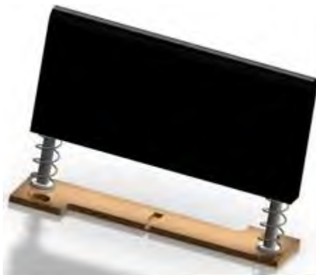
Figure 2.4 Polyethylen sliders, guided and springs details
