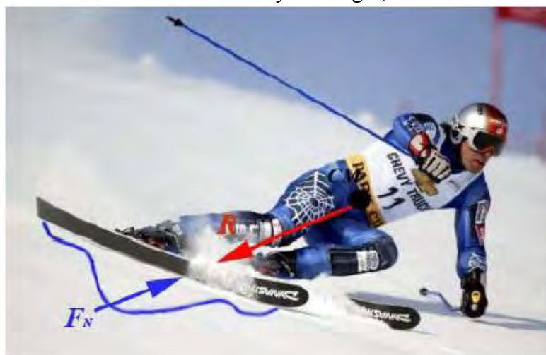
Figure 1.4 Resultant skier force R and ground reaction force F_N
