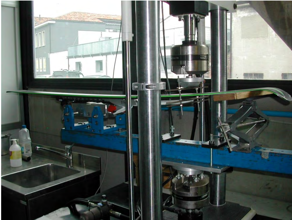
Figure 3.20 MTS machine configuration during arm stiffness characterization in DII
