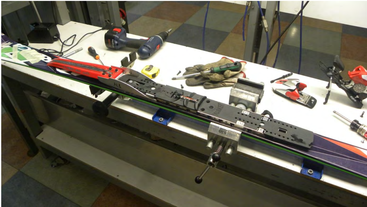
Figure 2.9 Ski without binding system with the elastic compensation superstructure
