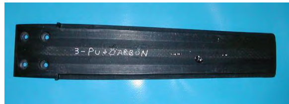
Figure 3.16 PU + C, polyurethane with carbon layers
