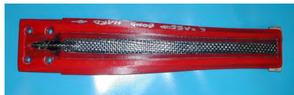
Figure 3.17 CHB, polyurethane with carbon visible layer
