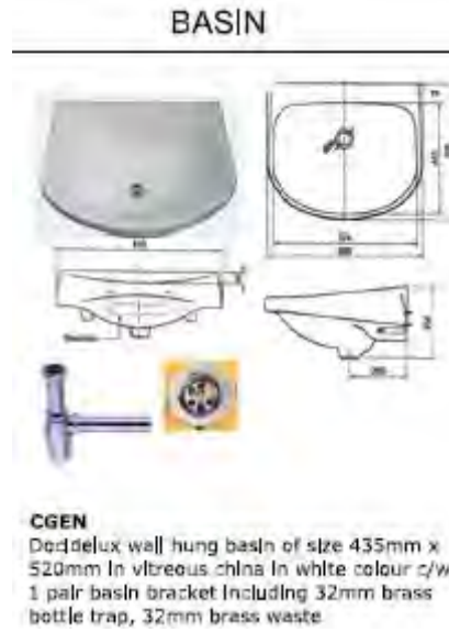
Figure 24 - Washbasin appearing in sanitary schedule.
