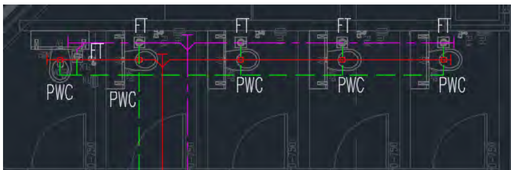
Figure 3 – Example of missing diameters.
