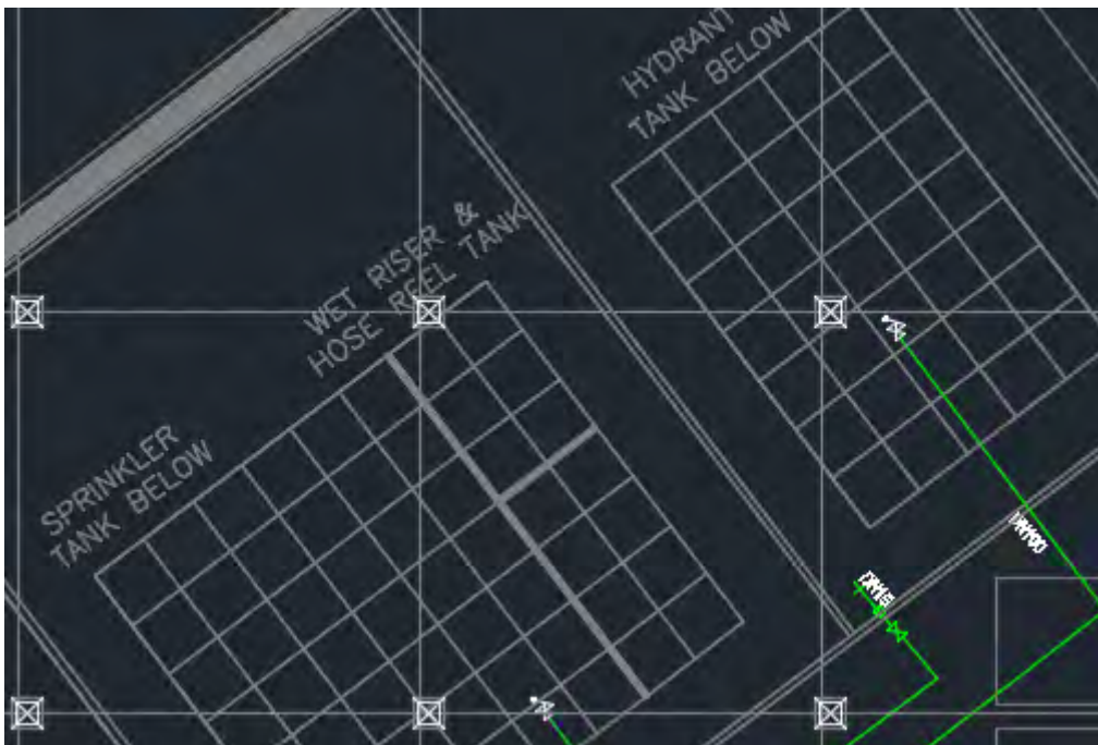
Figure 25 - Pillars passing through FRP water tanks.
