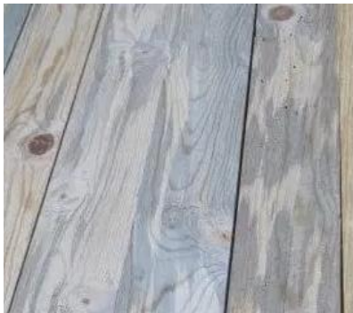
Figure 1.8. Defects in wood caused by fungi (theconstructor.org,2022)
