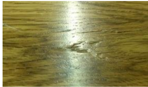
Figure 1.13. Torn grain (theconstructor.org,2022)
