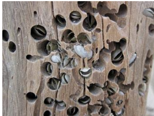
Figure 1.10. Marine borers in wood (theconstructor.org,2022)
