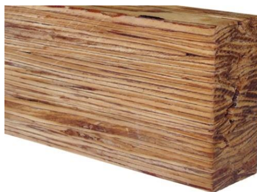
Figure 1.20. Parallel strand lumber ( https://www.dataholz.eu ,2022).
