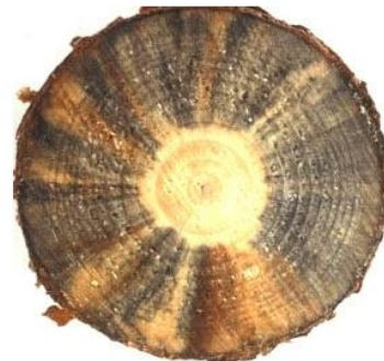
Figure 1.8. Defects in wood caused by fungi (theconstructor.org,2022)
