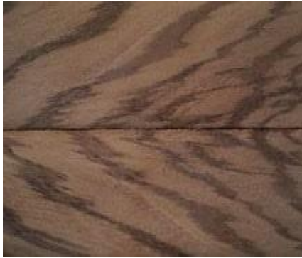
Figure 1.12. Diagonal grain (theconstructor.org,2022)
