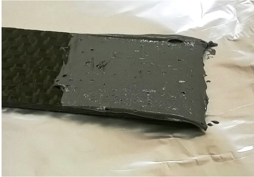
Figure 2.2: Epoxy resin on a carbon fiber plate after heat and vacuum treatment. Note the bubbles that come up to the surface
