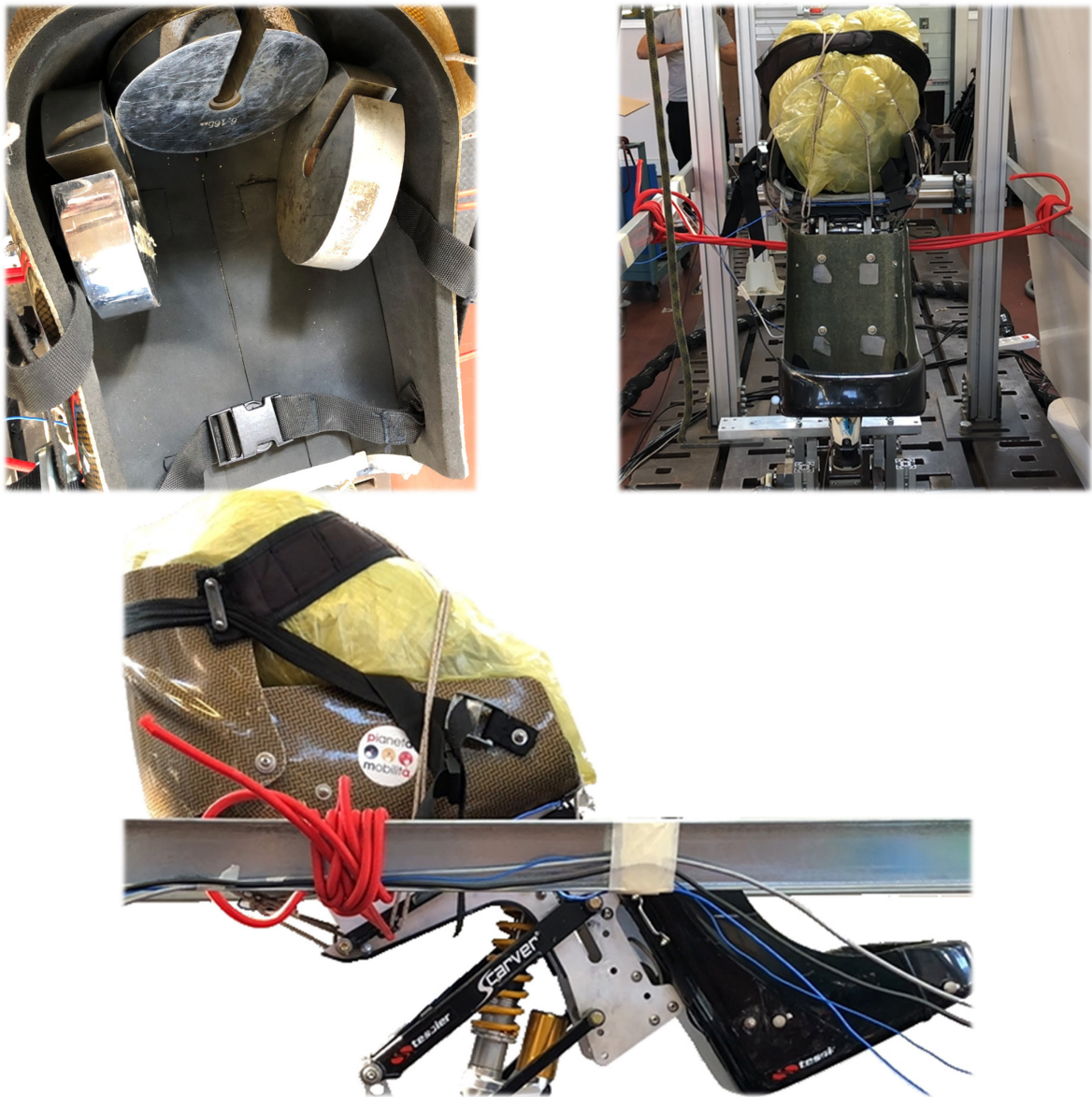
Figure 12.29: Weights and sandbag strapped in the seat
