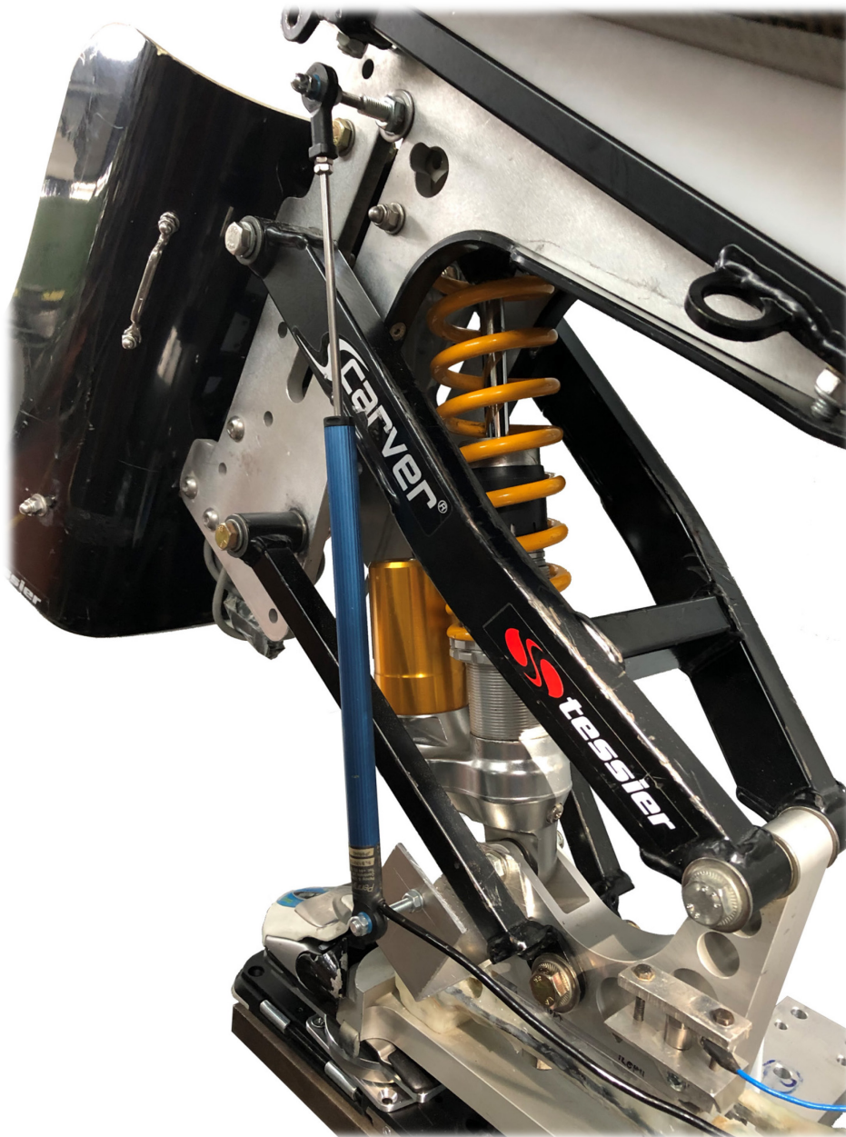
Figure 12.7: View of the potentiometer fixed on the monoski
