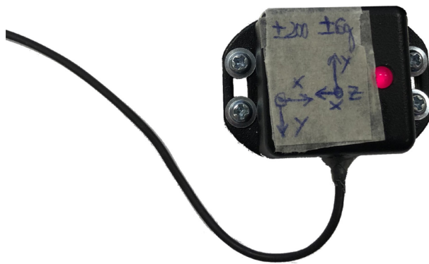
Figure 8.1: Accelerometers and reference system of each
