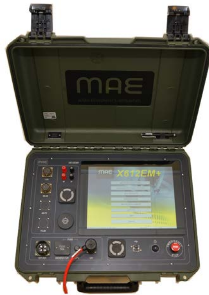
Fig. 2.8: Geo-resistivimetro multicanale X612EM (MAE Advanced Geophysics Instruments).
