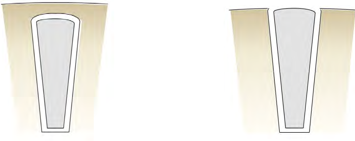
Figure 3.10: Close rotor slot shape (right) and open rotor slot shape (left).
