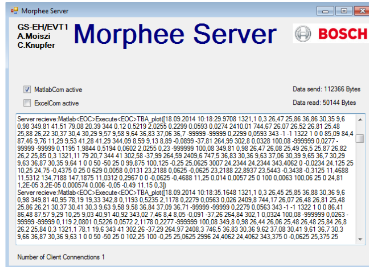
Figure 5.3: Server interface receiving measurements by the client.[Bosb]
