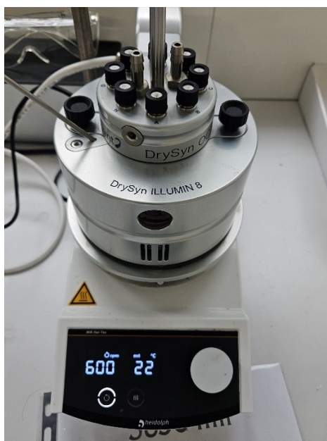
Figure 2.3 DrySyn Illumin8 reactor above the magnetic hotplate
