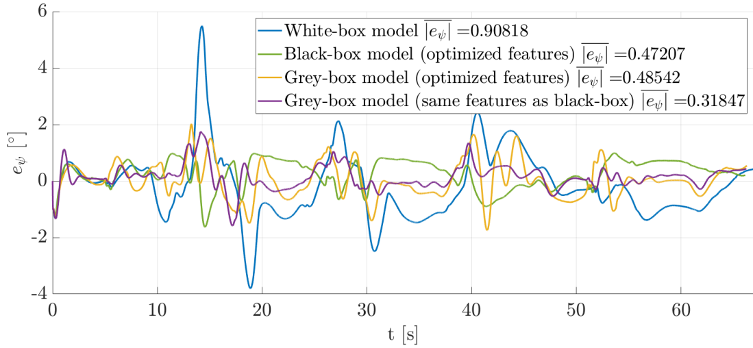
(b) Evolution of the yaw trajectory error e_\psi .
