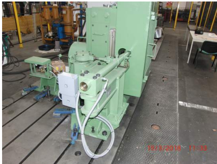
Figure 1.1: Back of the brushless eccentric deviator.
