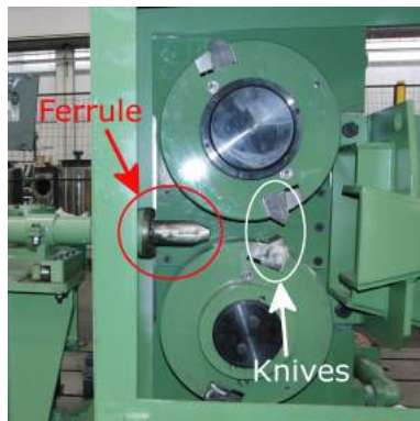
(a) End on the deviator with its ferrule and shear of the plant.
