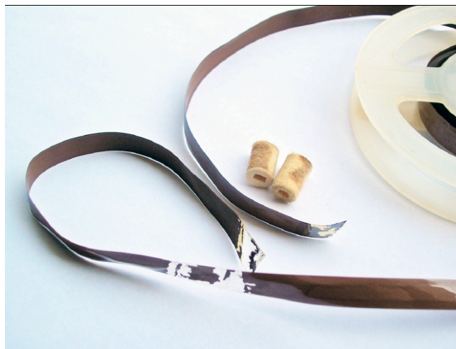
Fig. 7. reel no. 26: magnetic paste detachment from the support on splices of adjacent layers, caused by the use of common adhesive tape, unsuitable for magnetic tape splices. The glue has now dried and come away. The two cylinders are the anti-static cleaning felt pads, which have absorbed the detached powdered magnetic oxide.
