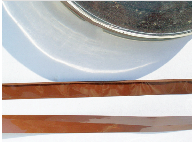
Fig. 4. reel no. 18 before cleaning, with deep tape folding for several metres at the beginning.
