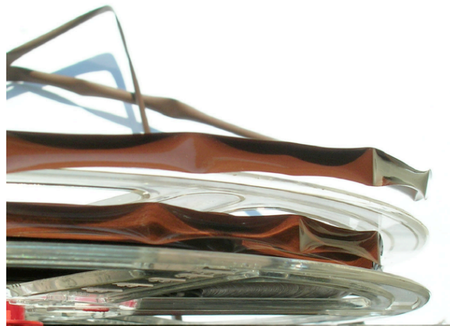
Fig. 3. reel no. 15: the initial 2 metres are badly damaged, with folding, undulations and structural fragility.
