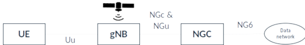
Figure 2.6: 5G NR NTN architecture for access network based on satellites with on-board gNB payload [8]
