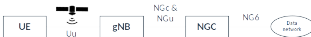
Figure 2.5: 5G NR NTN architecture for access network based on satellites with bent pipe payload [8]
